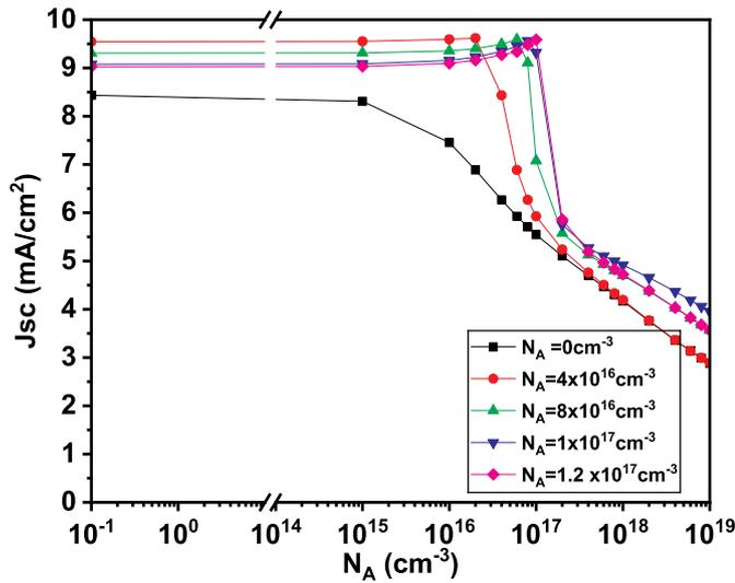
Fig. 3. Variation of the short circuit current density of P3HT:IC<sub>60</sub>BA based solar cell as function of  $N_D$  for different values of  $N_A$ .
