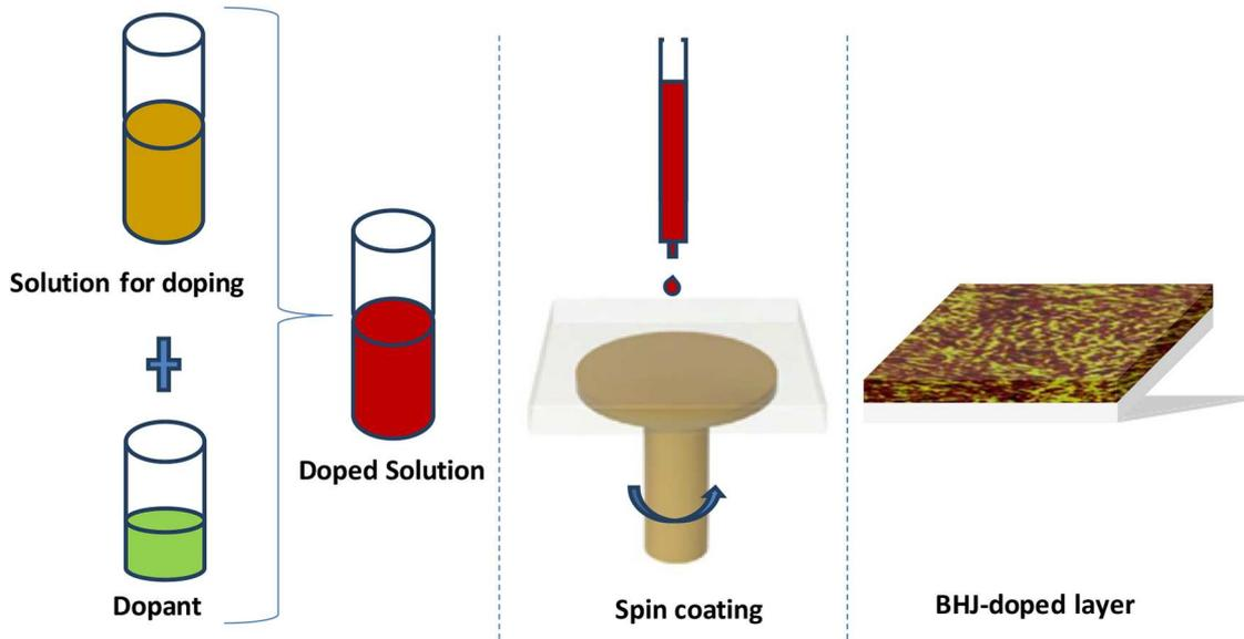
Fig. 2. Chemical method doping: solution-processing through liquid phase.
