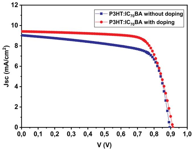
Fig. 8.  $J-V$  characteristics of the OPV solar cell based on P3HT: IC<sub>70</sub>BA; without doping (blue color) and with doping (red color).
