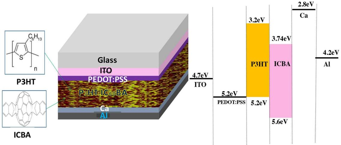
Fig. 1. Organic solar cell based on ITO/PEDOT:PSS/P3HT:IC<sub>60</sub>BA/Ca/Al structure [39].
