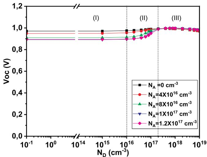
Fig. 4. Evolution of the open circuit voltage for P3HT:IC<sub>60</sub>BA based solar cell as function of  $N_D$  for different values of  $N_A$ .
