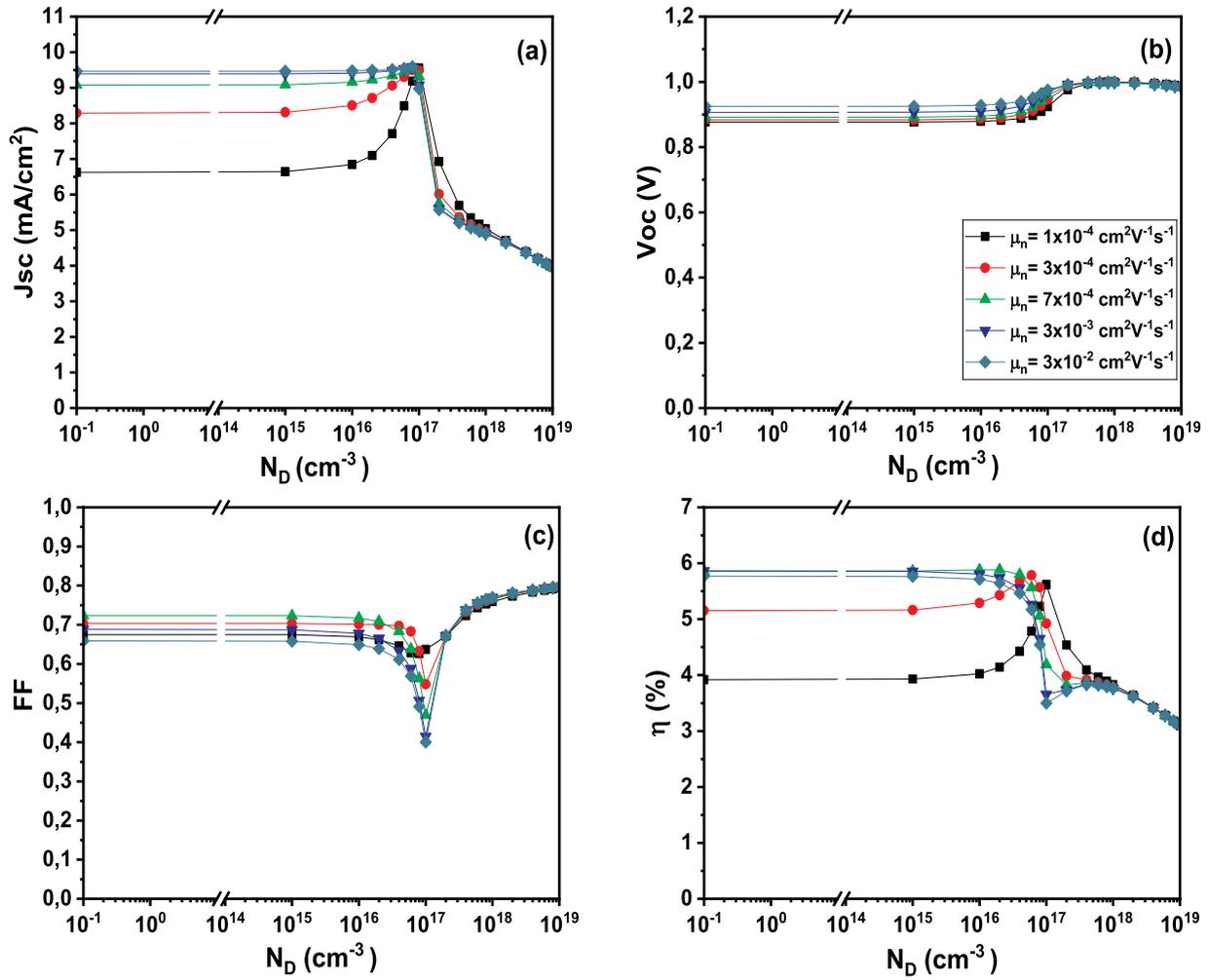
Fig. 7. The effect of N-type doping concentration  $N_D$  on the performances of P3HT: IC<sub>60</sub>BA based solar cell for different electron mobilities.
