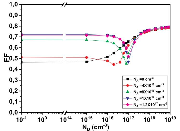
Fig. 5. Variation of the fill factor of P3HT:IC<sub>60</sub>BA based solar cell as function of  $N_D$  for different values of  $N_A$ .
