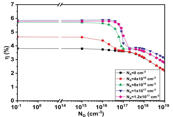
Fig. 6. Evolution of the efficiency of the P3HT:IC<sub>60</sub>BA based solar cell as function of  $N_D$  for different values of  $N_A$ .
