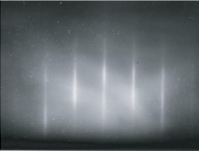
**Fig. 2.** A typical RHEED pattern observed for an  $\text{La}_{0.7}\text{Sr}_{0.3}\text{MnO}_{3-\delta}$  epitaxial thin film grown on STO (100) at  $820^\circ\text{C}$ .
