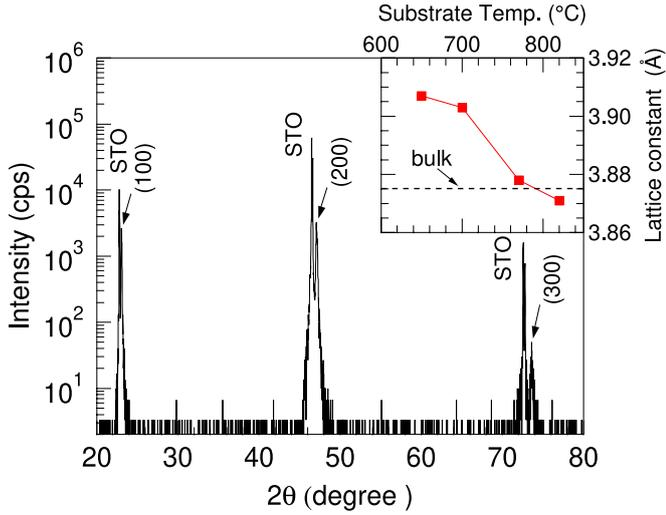
**Fig. 1.** A typical XRD pattern observed for an  $\text{La}_{0.7}\text{Sr}_{0.3}\text{MnO}_{3-\delta}$  epitaxial thin film grown on STO (100) at  $820^\circ\text{C}$ . The inset plots the lattice constant observed vs the substrate temperature.
