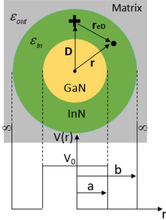
**Fig. 1.** Schematic representation of core/shell Quantum Dot structure.
