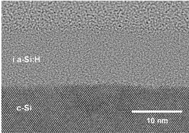
**Fig. 4.** TEM cross-sectional image for the sample with  $\sim 12$  nm thick a-Si:H layers prepared with a mesh temperature ( $T_{\text{mesh}}$ ) of  $370^\circ\text{C}$ .
