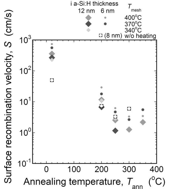
**Fig. 3.** Surface recombination velocity ( $S$ ) versus post-deposition annealing temperature ( $T_{ann}$ ) for samples with 6 or 12 nm thick a-Si:H passivation layers prepared with different mesh temperature ( $T_{mesh}$ ). Note that the thickness of the sample prepared without gas-heating was exceptionally ~8 nm.
