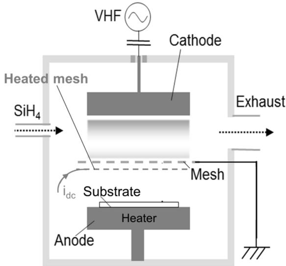
**Fig. 1.** Our triode-type PECVD reactor with gas-heating system.
