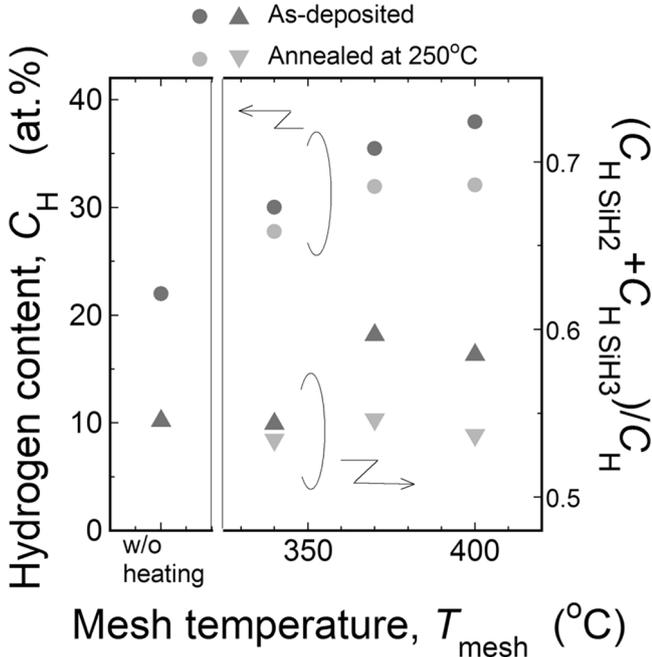
**Fig. 2.** Total bonded hydrogen content ( $C_H$ ) and  $(C_{H_{SiH2}} + C_{H_{SiH3}})/C_H$  versus mesh temperature ( $T_{mesh}$ ), where the  $C_{H_{SiH2}}$  and the  $C_{H_{SiH3}}$  are hydrogen contents in Si=H2 and Si≡H3, respectively, for as-deposited or 250°C-annealed samples with ~12 nm thick a-Si:H layers. The data for an as-deposited sample with ~8 nm thick a-Si:H layers prepared without gas-heating is also shown on the left side of the figure.
