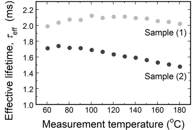
**Fig. 5.** Temperature-dependence of the minority carrier effective lifetime ( $\tau_{\text{eff}}$ ) for Sample (1) prepared with gas-heating turned on before deposition starts and for Sample (2) prepared with gas-heating turned on after deposition starts.
