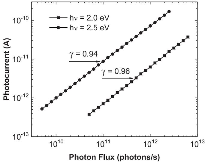
**Fig. 3.** Variation of *ac* photocurrent component with incident flux of 2 and 2.5 eV photons. The chopping frequency is 6 Hz.
