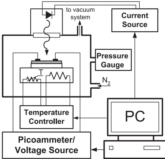
**Fig. 1.** Schematic diagram of a photoconductivity measurement setup.
