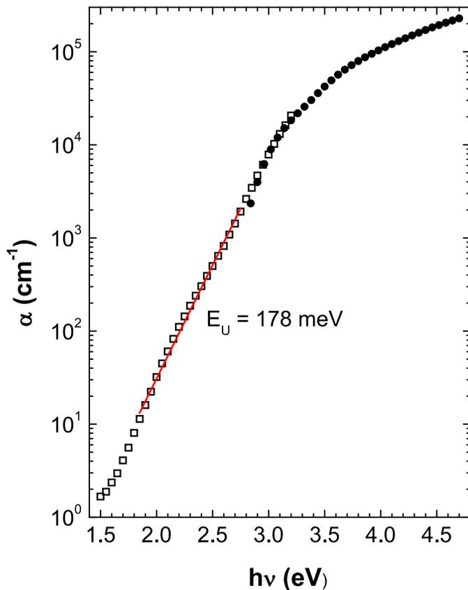
**Fig. 4.** Absorption coefficient  $\alpha$  versus photon energy  $h\nu$  derived from photoconductivity (squares) and transmission (circles) measurements.
