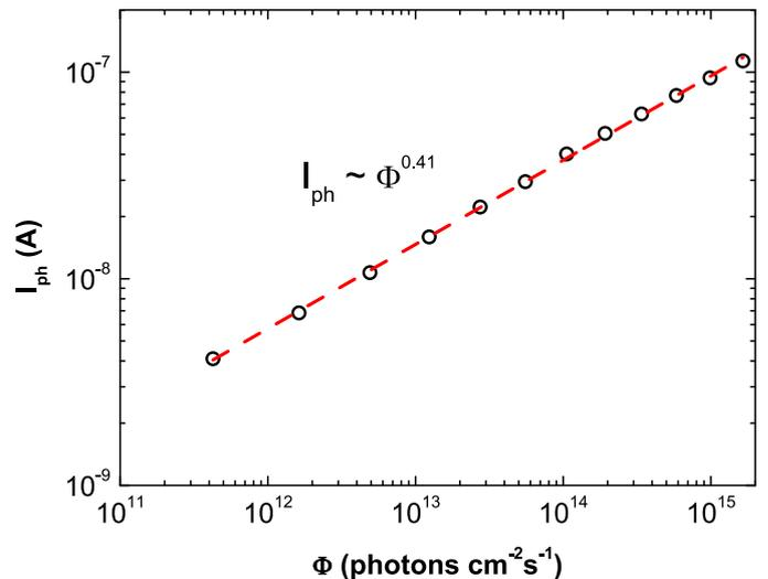
Fig. 8. Steady-state photocurrent as a function of photon flux density  $\Phi$ .
