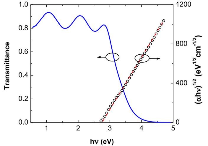
**Fig. 2.** Transmission spectrum and Tauc's plot.
