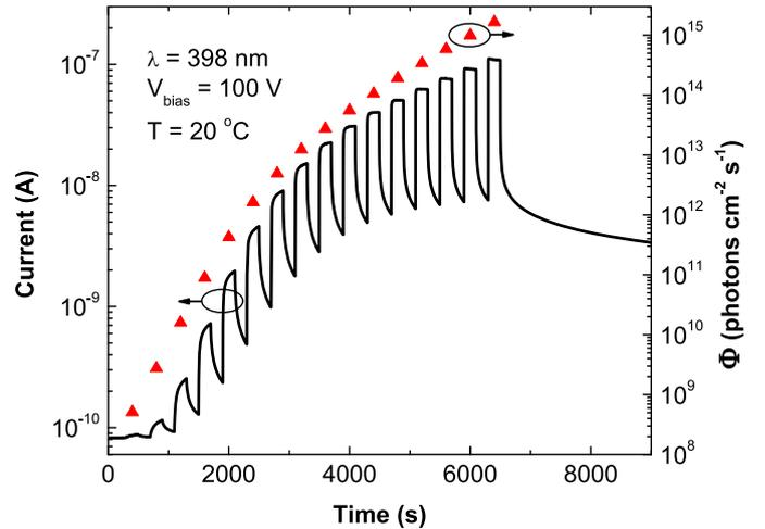
Fig. 7. Photoresponse to 200s light pulses. The photon flux density is shown for each pulse (triangles).
