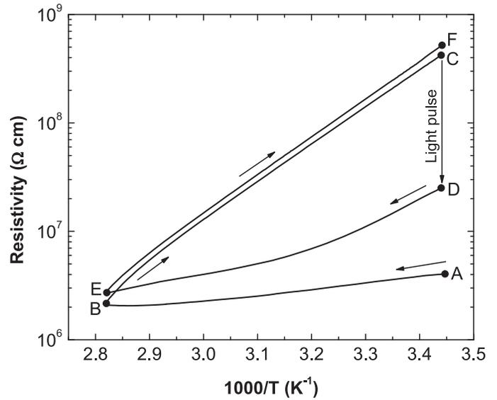
**Fig. 5.** Temperature dependence of resistivity of the  $\text{In}_{1-x-y}\text{S}_x\text{F}_y$  film.
