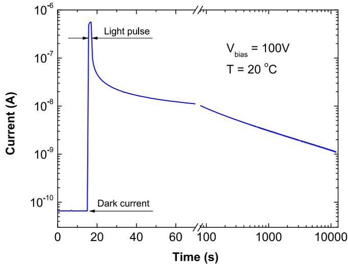
Fig. 6. Photoresponse on 2s light pulse.
