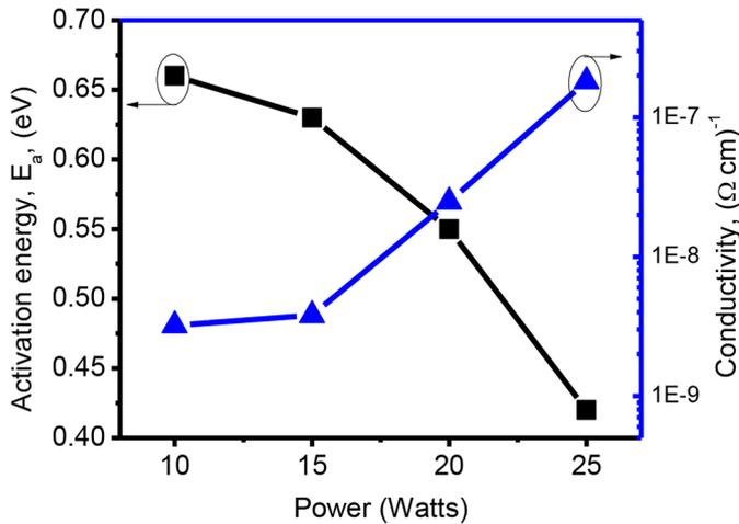
**Fig. 6.** Activation energy ( $E_a$ ) and dark conductivity both as function of deposition RF-power.
