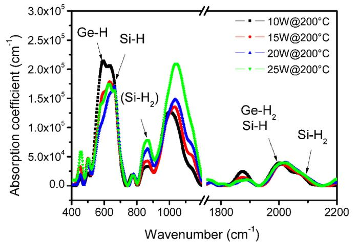
Fig. 3. IR spectra of nc-SiGe:H thin films deposited at different RF-power.
