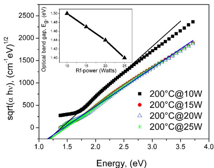
**Fig. 5.** Optical band gap obtained from Tauc method of nc-SiGe:H thin films. Inset of figure shows the optical band gap as a function of deposition RF-power.
