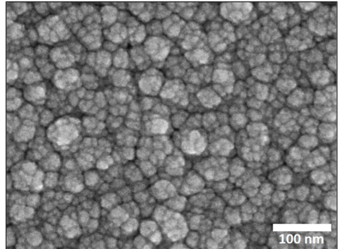
Fig. 2. FE-SEM image of the surface of a nc-SiGe:H film.
