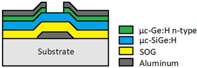
Fig. 1. Cross section of nc-SiGe:H TFT-BG fabricated.
