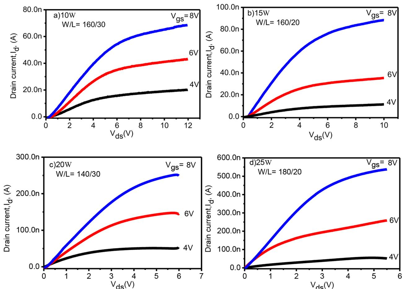
Fig. 8. (a)–(d) Output characteristic of TFT with W/L = 160/30, 160/20, 140/30 and 180/20 of nc-SiGe:H TFTs.
