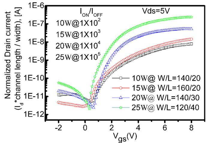
**Fig. 7.** Normalized transfer characteristics in the saturation region ( $V_{ds} = 5V$ ) of TFT with different widths and channel lengths.
