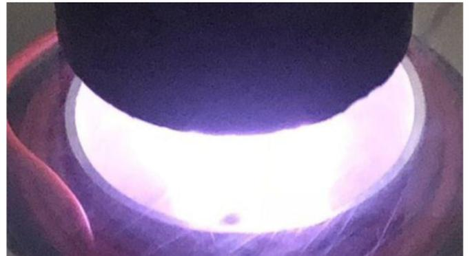
Fig. 6. Glow discharge under weak magnetic field.
