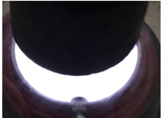
Fig. 5. Glow discharge under high-intensity magnetic field.
