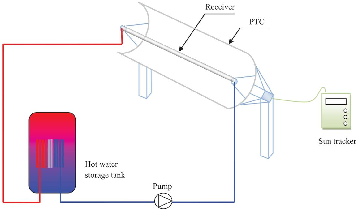
**Fig. 1.** Scheme of the thermal energy producing system driven by PTC.
