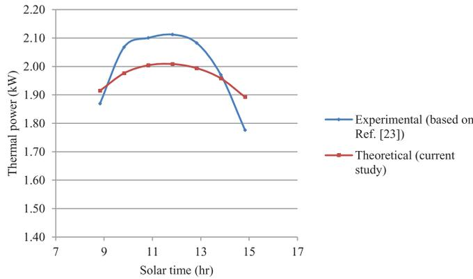
**Fig. 10.** Hourly variation of thermal power on June 21.
