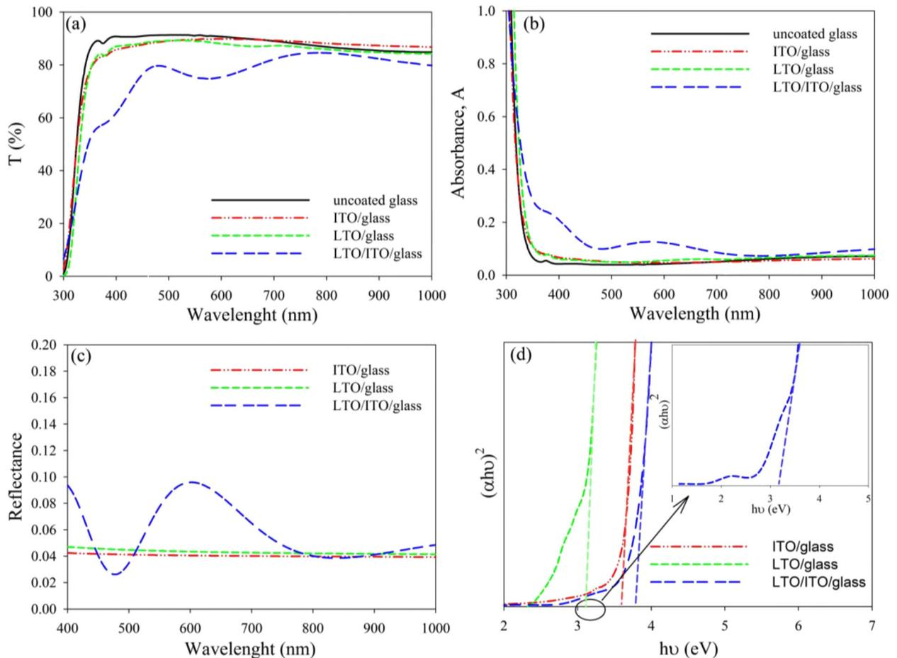
**Fig. 2.** (a) Transmittance, (b) absorbance, (c) reflectance spectra of the LTO thin film deposited on ITO/glass substrate and (d) Tauc plot of  $(\alpha hv)^2$  vs.  $hv$  to obtain the optical band gap energy.
