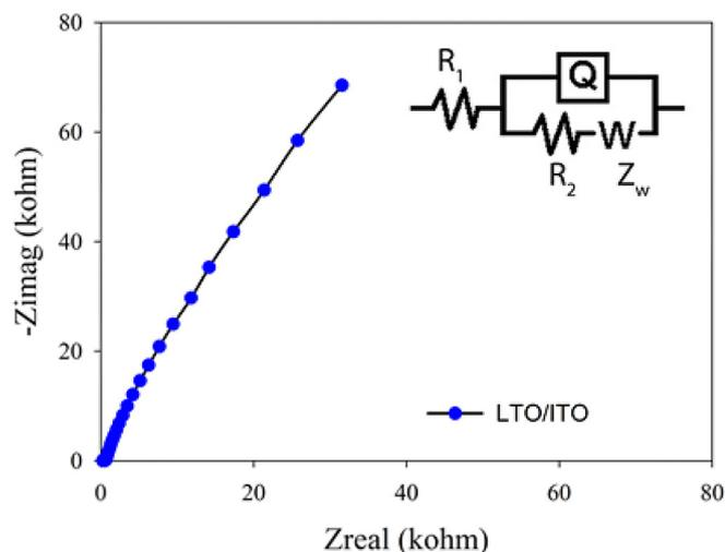
**Fig. 3.** The impedance spectrum and Randles circuit obtained from the impedance analysis.
