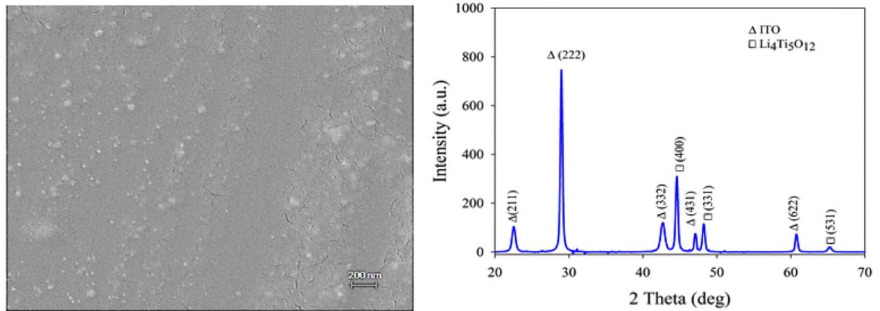
**Fig. 1.** (a) Top view FESEM image and (b) XRD pattern of the LTO thin film deposited on ITO/glass substrate.
