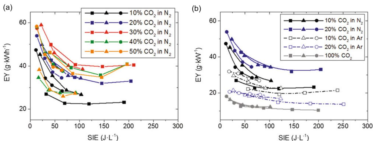
**Fig. 6.** Energy yield at different concentration of CO<sub>2</sub> in N<sub>2</sub> (a) as well as N<sub>2</sub> and Ar (b). Squares are related to 100 L h<sup>-1</sup>, triangles to 200 L h<sup>-1</sup> and circles to 300 L h<sup>-1</sup> flowrate.
