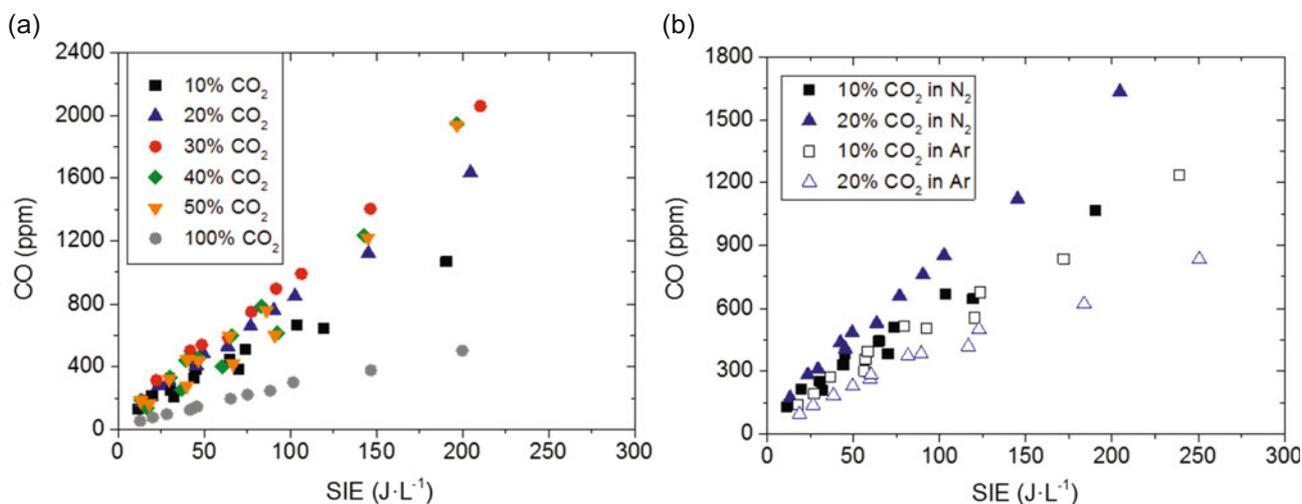
Fig. 3. CO production at different concentration of CO<sub>2</sub> in N<sub>2</sub> and Ar.
