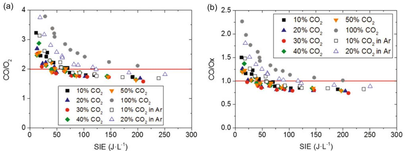
**Fig. 5.** (a)  $\text{CO}/\text{O}_2$  ratio and (b)  $\text{CO}/\text{O}_x$  ratio depending on SIE and gas composition. The red lines mark the corresponding stoichiometric values.
