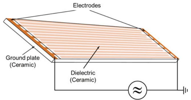
**Fig. 1.** Schematic representation of the coplanar discharge arrangement (the upper dielectric layer is here only for explanatory purpose transparent).
