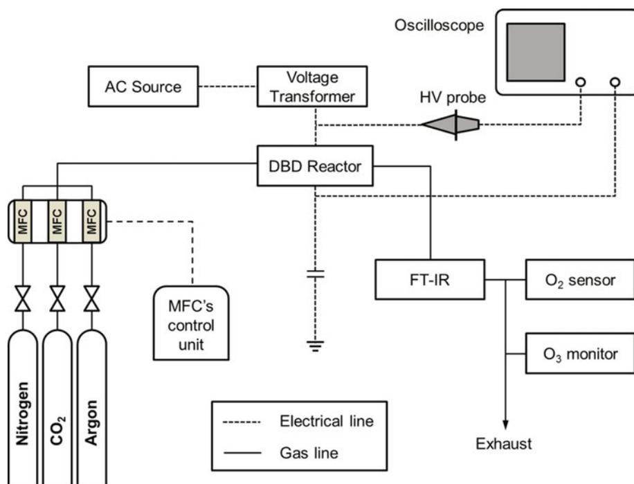
Fig. 2. Schematic representation of the experimental setup.
