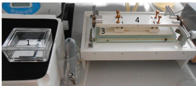
**Fig. 2.** DCBSD reactor for inactivation of *E. coli* on the contaminated PTFE surface: 1 – contaminated PTFE samples, 2 – sterile forceps, 3 – DCBSD plasma system, 4 – movable sample holder.
