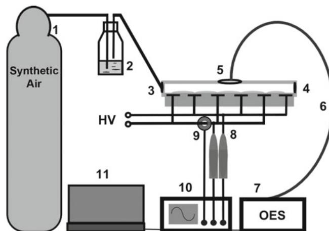
**Fig. 1.** The scheme of the measurement of DCSBD parameters: 1 – synthetic air, 2 – bubbler with distilled water, 3 – gas input, 4 – gas output, 5 – quartz glass window, 6 – optical fiber, 7 – spectrometer, 8 – high voltage probes, 9 – Rogowski's coil, 10 – oscilloscope, 11 – computer.
