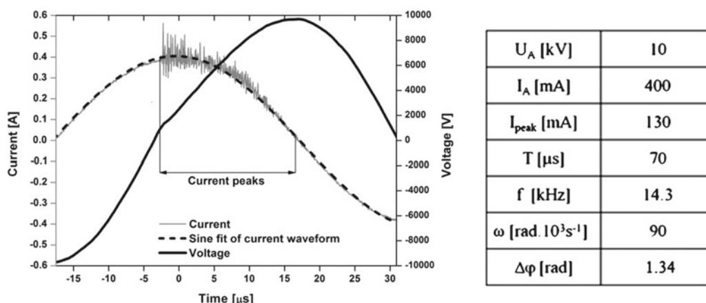
**Fig. 3.** Voltage/current waveforms and discharge current peaks of DCSBD plasma generated in ambient air at input power 400 W and characteristic parameters obtained using sine simulation of voltage/current waveforms.
