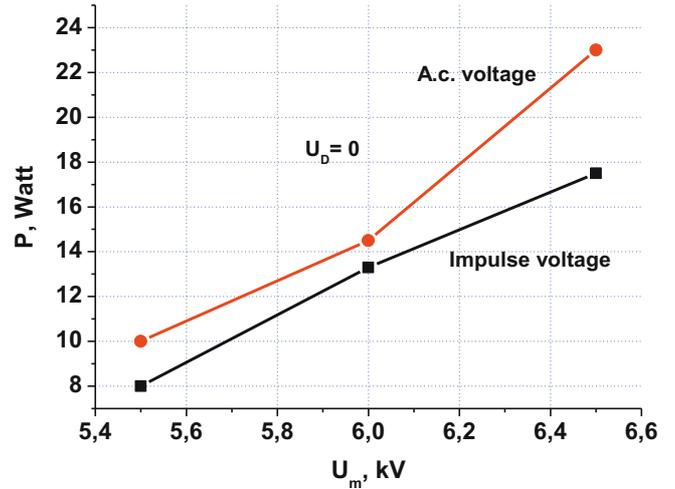
**Fig. 7.** Active power of the surface discharge under impulse and a.c. voltage for  $U_D = 0$ . Values of  $U_m$  correspond to impulse voltage amplitude and to p/p values of the a.c. voltage.
