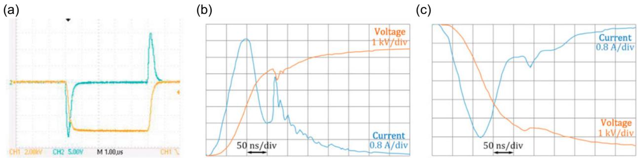
Fig. 2. Typical oscillograms of the voltage and current of surface discharge.
