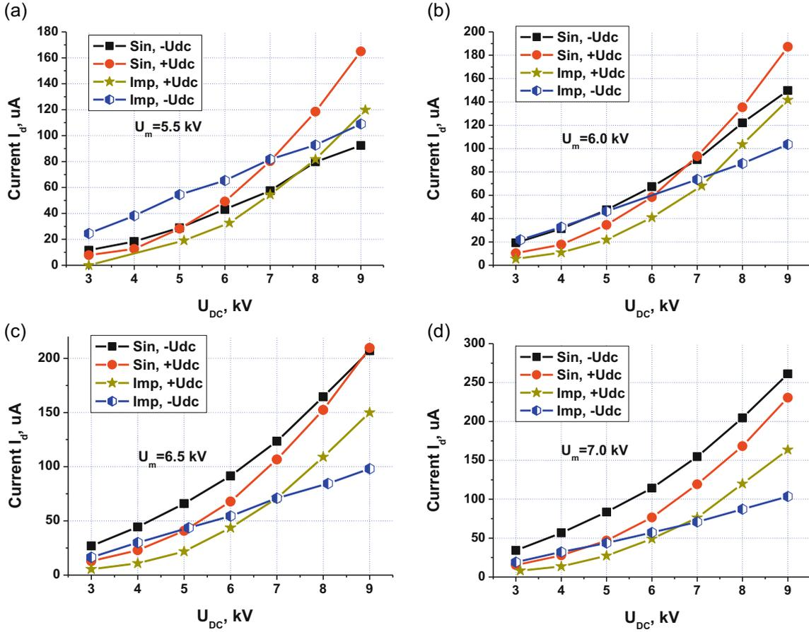
**Fig. 8.** Comparison of “extracted” currents as a function of  $U_{DC}$  for different positive impulse voltage amplitudes and different values of a.c. voltage (peak-to-peak values).
