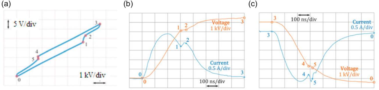
**Fig. 5.** Correlation between the Volt-Coulomb characteristic of impulse surface discharge and voltage and impulse current curves. (a)  $U - Q$  curve; (b) current and voltage curves at the front of the voltage impulse; (c) current and voltage curves at the falling part of the voltage impulse.
