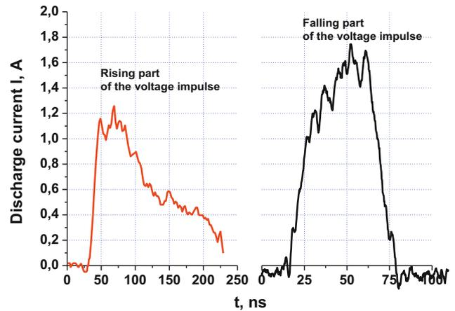
Fig. 3. Examples of current impulses of surface discharge at the rising and falling parts of the applied voltage impulse.
