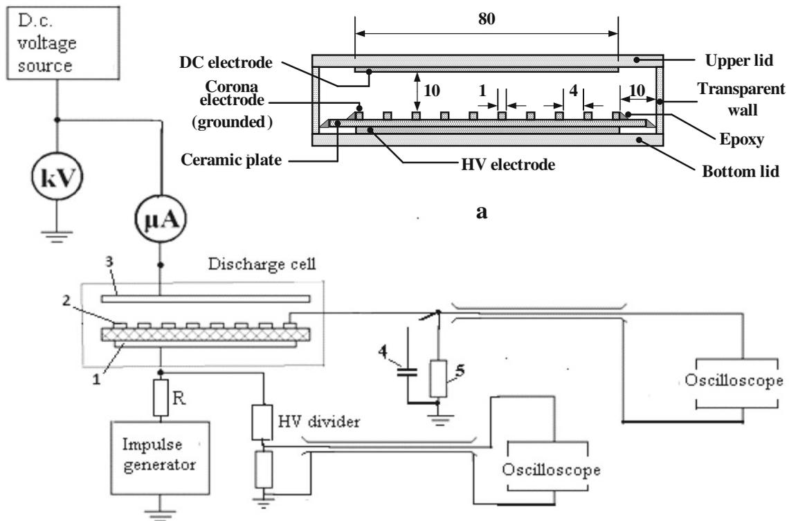
**Fig. 1.** Electric circuit with discharge cell (a): 1–3 – electrodes, 4 – measuring capacitor  $C_m$ ; 5 – measuring resistor  $R_m$ ;  $R$  – series resistor of impulse generator. All dimensions are in mm.
