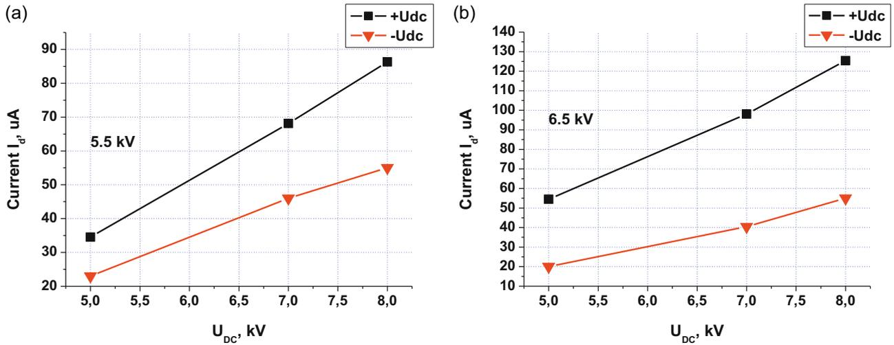
**Fig. 10.** Comparison of “extracted” currents for  $U_m = 5.5$  kV (a) and  $U_m = 6.5$  kV (b) and for different values and polarity of  $U_{DC}$ .
