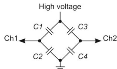
Fig. 4. Electric circuit to measure the Volt-Coulomb characteristic.
