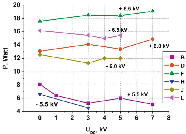
**Fig. 6.** Dependence of active power  $P$  of impulse surface discharge on the positive d.c. potential  $U_{DC}$  of the third electrode. Amplitude values ( $U_m$ ) and polarity of the voltage impulse are given in the figure.
