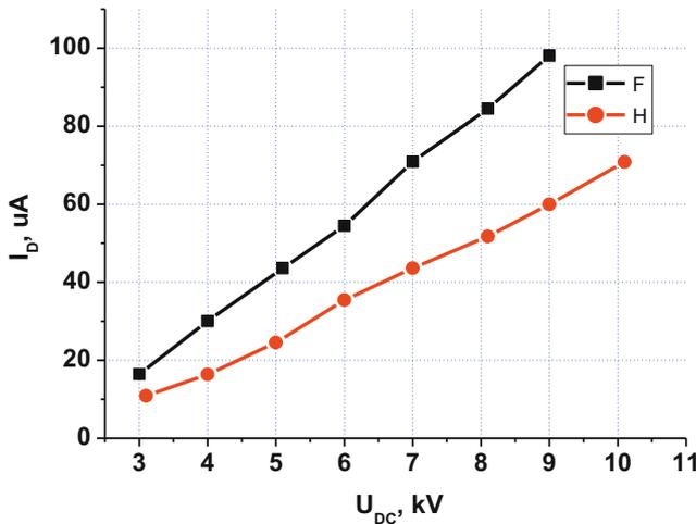
**Fig. 11.** Comparison of “extracted” currents for different distances from barrier surface to third electrode.  $U_m = 6.5$  kV, curve  $F$  is for  $d = 1$  cm, curve  $G$  is for  $1.4$  cm.
