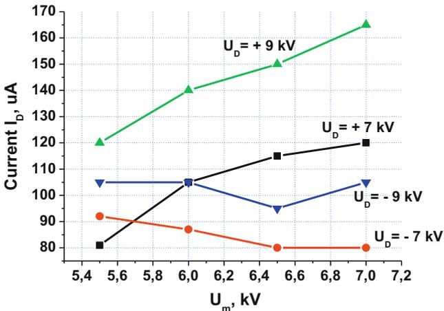
**Fig. 9.** Comparison of “extracted” currents as a function of positive impulse voltage amplitudes for different values and polarity of the  $U_{DC}$ .
