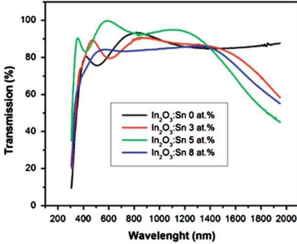
**Fig. 4.** Optical transmittance spectra of ITO films as a function of Sn-doping levels.
