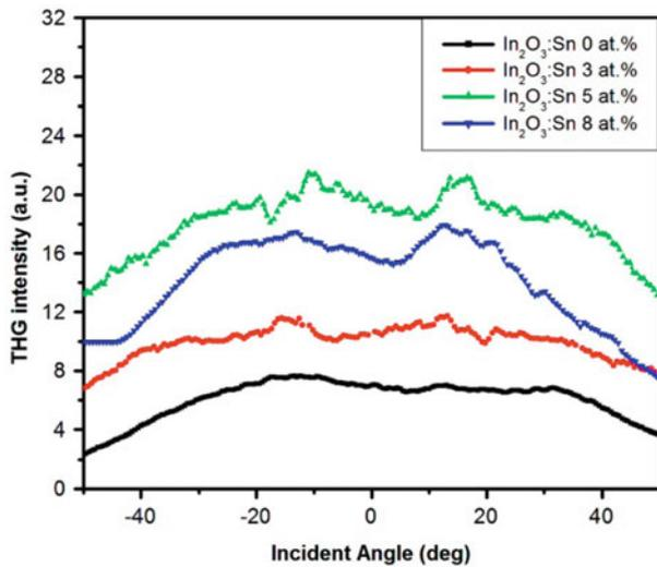
**Fig. 7.** Normalised third harmonic response of undoped and Sn-doped In<sub>2</sub>O<sub>3</sub> thin films.
