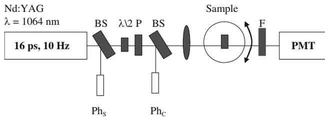
**Fig. 2.** THG experimental setup,  $\text{Ph}_s$ : synchronisation photodiode,  $\text{Ph}_c$ : control photodiode,  $\lambda/2$ : half wave plate, BS: beam splitter, P: polariser, F: transmitting filter at  $355\text{ nm}$ , PMT: photomultiplier tube.
