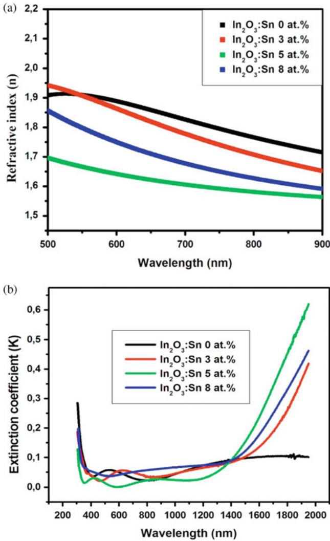
**Fig. 6.** Wavelength dependence of (a) the refractive index and (b) the extinction coefficient of ITO films with different Sn doping concentrations.
