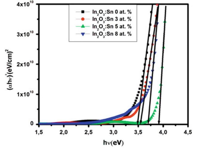
**Fig. 5.** Variation of optical band gap energy of ITO films with different Sn doping concentrations.
