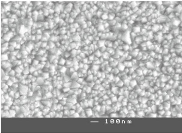
**Fig. 1.** SEM images of  $\text{In}_2\text{O}_3:\text{Sn}$  (5 at.%) prepared at  $500^\circ\text{C}$ .
