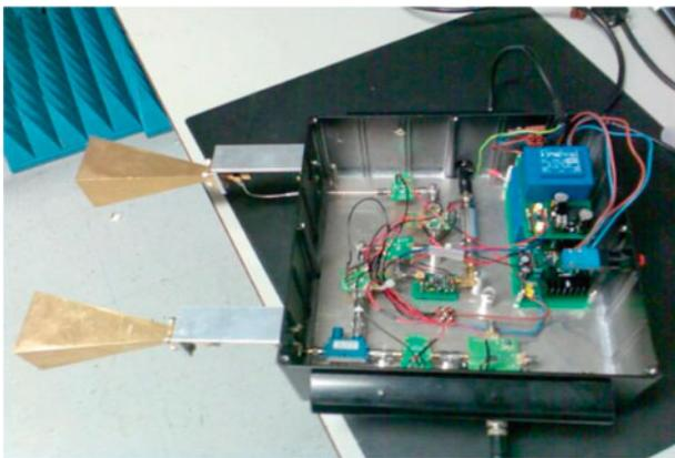
Fig. 6. FMCW radar [21].
