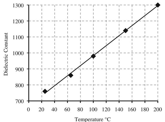
Fig. 3. Permittivity of the sensitive material versus temperature.
