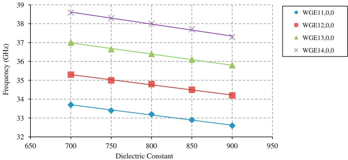
**Fig. 4.** Frequencies versus dielectric constant for WGE<sub>11,0,0</sub>, WGE<sub>12,0,0</sub>, WGE<sub>13,0,0</sub> and WGE<sub>14,0,0</sub> modes.
