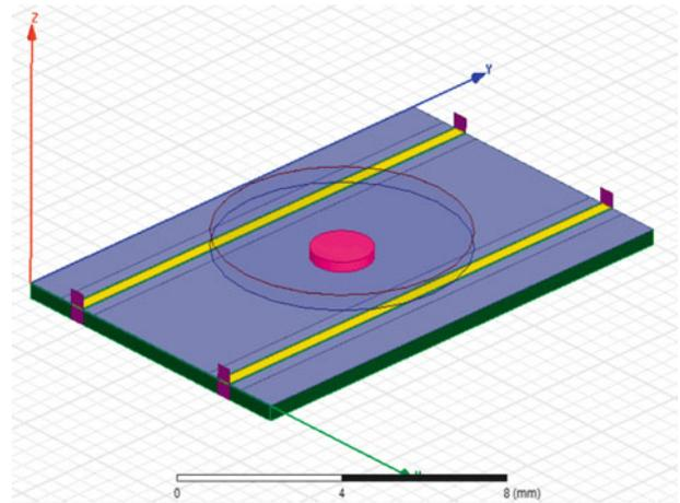
Fig. 1. Topology of the proposed sensor.
