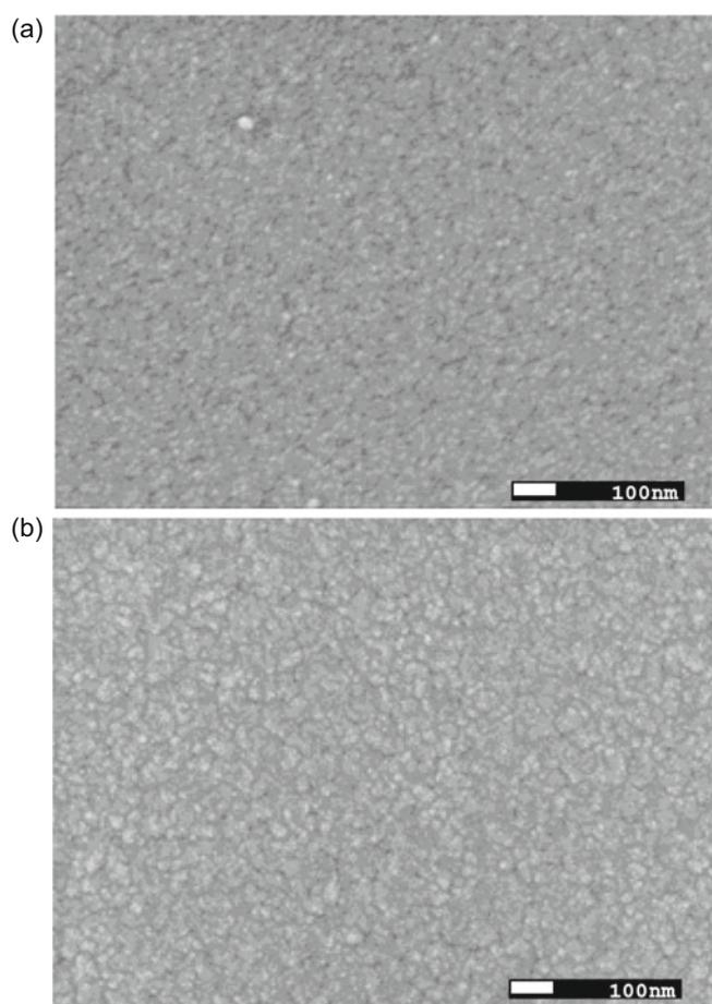
**Fig. 2.** Scanning electron microphotography showing the surface morphology of (a) Cu (12 nm)/MoO<sub>3-x</sub> (20 nm) and (b) Cu (12 nm)/MoO<sub>3-x</sub> (20 nm)/Al (0.5 nm)/MoO<sub>3-x</sub> (10 nm).
