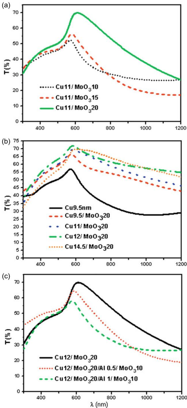
**Fig. 1.** Transmittance spectra of the glass/Cu/MoO<sub>3-x</sub> with different layer thickness.
