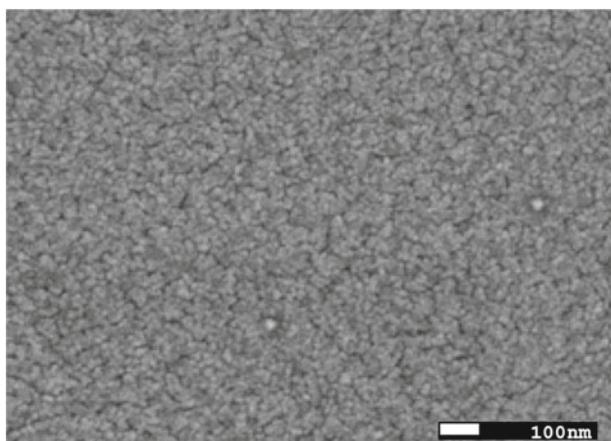
**Fig. 3.** SEM visualization of the surface of glass/Cu/MoO<sub>3-x</sub> in the backscattering mode.
