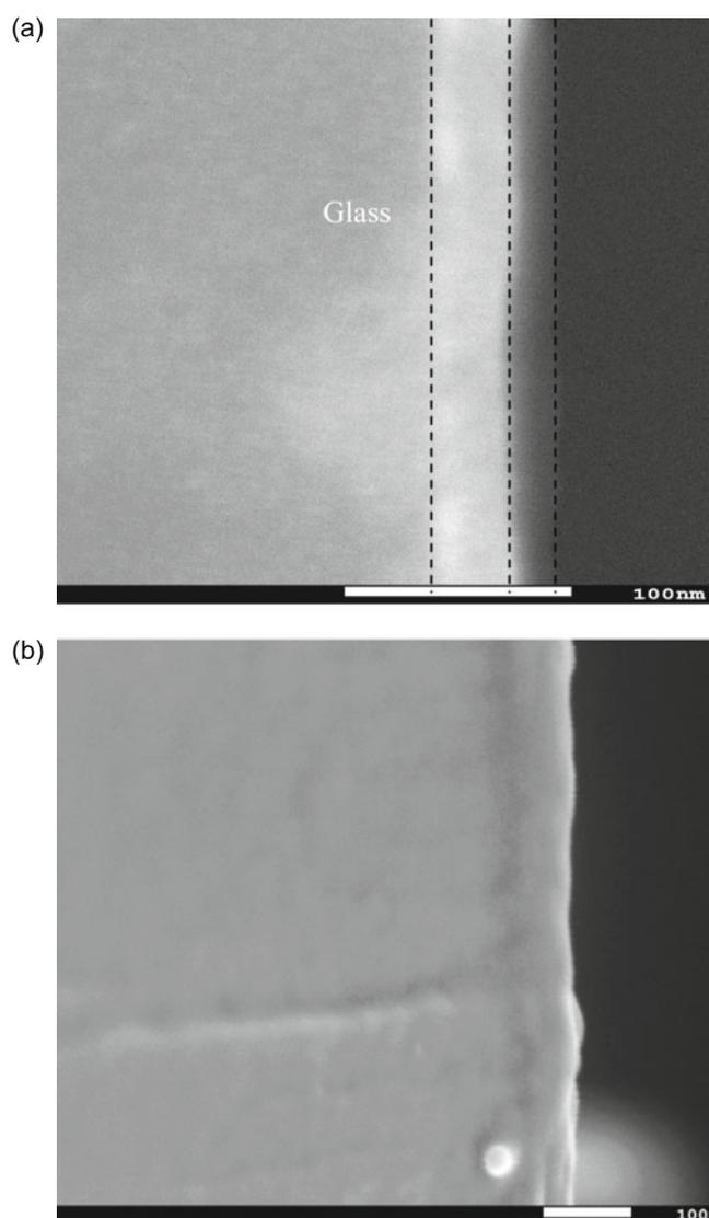
**Fig. 4.** Cross section visualization of Cu/MoO<sub>3-x</sub>/Al/MoO<sub>3-x</sub> (a) and Cu/MoO<sub>3-x</sub> (b).
