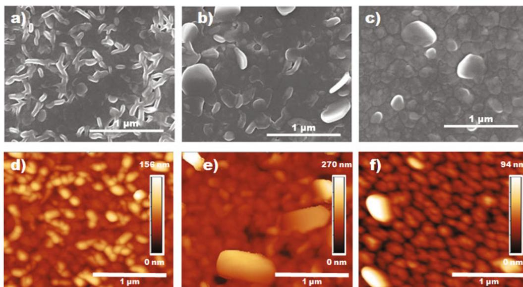
**Fig. 5.** SEM (a) and AFM (d) images of 5T layer deposited onto ITO/CuI. SEM (b) and AFM (e) images of 5T layer deposited onto ITO/MoO<sub>3</sub>/CuI. SEM (c) and AFM (f) images of 5T layer deposited onto ITO/MoO<sub>3</sub>.
