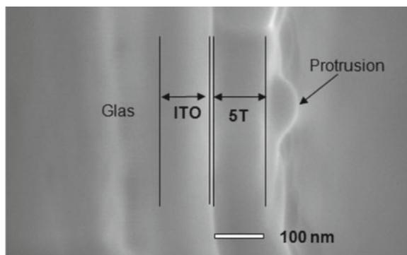
**Fig. 3.** Visualization of the cross section of 5T film (100 nm) deposited onto ITO/MoO<sub>3</sub>/CuI.
