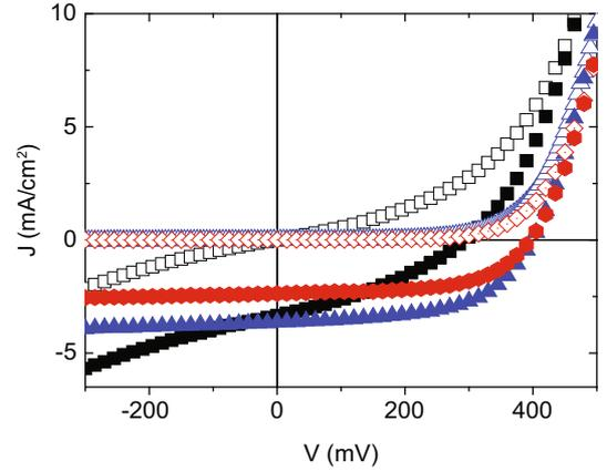
**Fig. 2.**  $J$ - $V$  characteristics of OPVCs using 5T as electron donor, and C<sub>60</sub> as acceptor, with different anode buffer layers: CuI (■), MoO<sub>3</sub>/CuI (▲) and MoO<sub>3</sub> (●) in the dark (full symbols) and under AM1.5 irradiation (open symbols).
