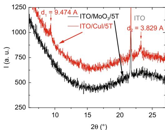
**Fig. 4.** X-ray diagrams of 5T layers deposited onto MoO<sub>3</sub> and CuI.
