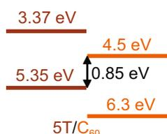
**Fig. 6.** Schematic band structure of the PHJ 5T/C<sub>60</sub>.
