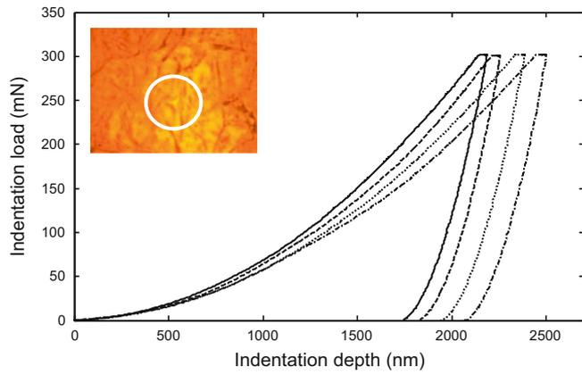
**Fig. 8.** Load-displacement curves of cold sprayed copper coating.
