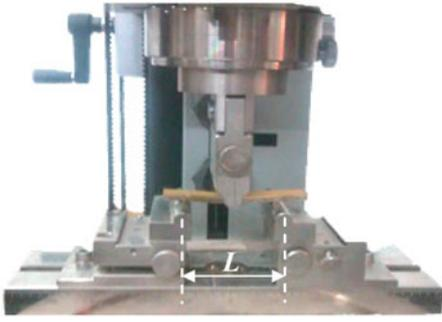
**Fig. 1.** Three point bending test set-up.
