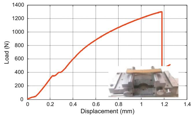
**Fig. 10.** Loading curve resulting from bending test, the inset is the fractured sample after bending test.
