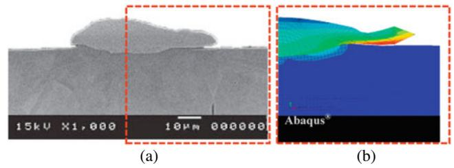
**Fig. 5.** Experimental [19] (a) and simulated morphologies of splats sprayed on SS substrate at 673 K.
