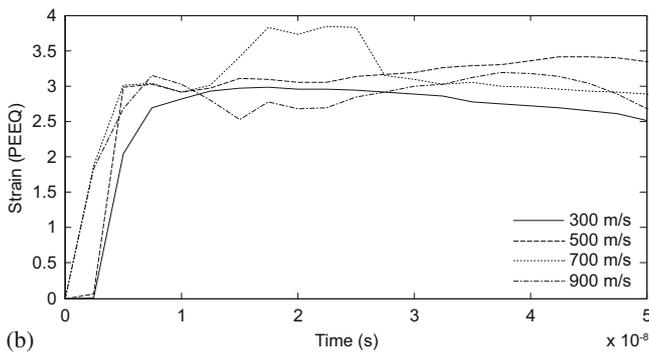
**Fig. 3.** Time evolution of effective plastic strain of copper particle under different particle velocities using Lagrangian (a) and ALE method (b).
