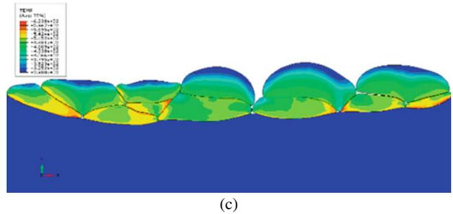
**Fig. 6.** Contours of the Von-mises stress (a), effective plastic strain (b) and temperature (c) of multi-particle impacting on the SS substrate at 250 ns modeled by ALE method.
