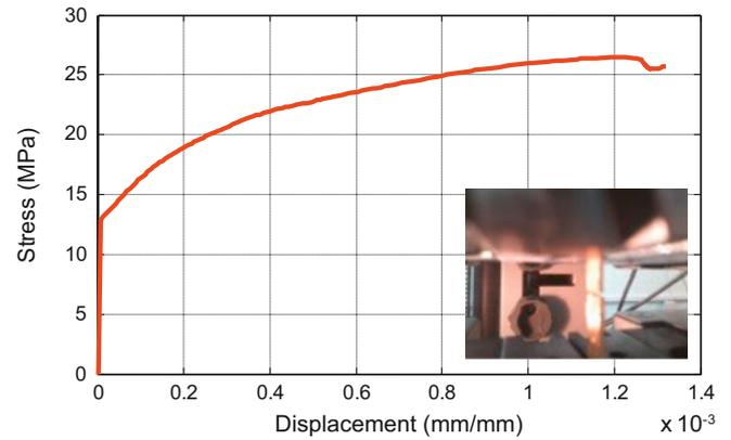
**Fig. 9.** A typical stress-strain curve obtained from copper coating tensile test. The inset is the fractured sample after tensile test.
