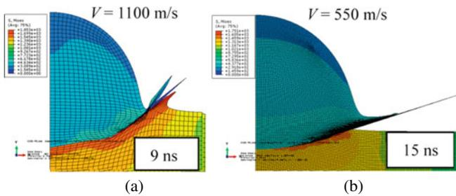
**Fig. 4.** Contours of Von-mises stress at the contact interface for the particle with the meshing size of 0.6 (a) and 0.1  $\mu\text{m}$  (b) modeled by Lagrangian method.
