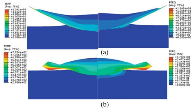
**Fig. 2.** Simulated contours of PEEQ and temperature using the Lagrangian (a) and ALE (b) methods.
