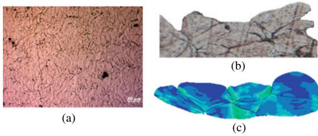
**Fig. 7.** SEM Micrograph of cold sprayed copper coating cross-section, (a) experimental, (b) calculated, (c) morphologies of particle deformed.
