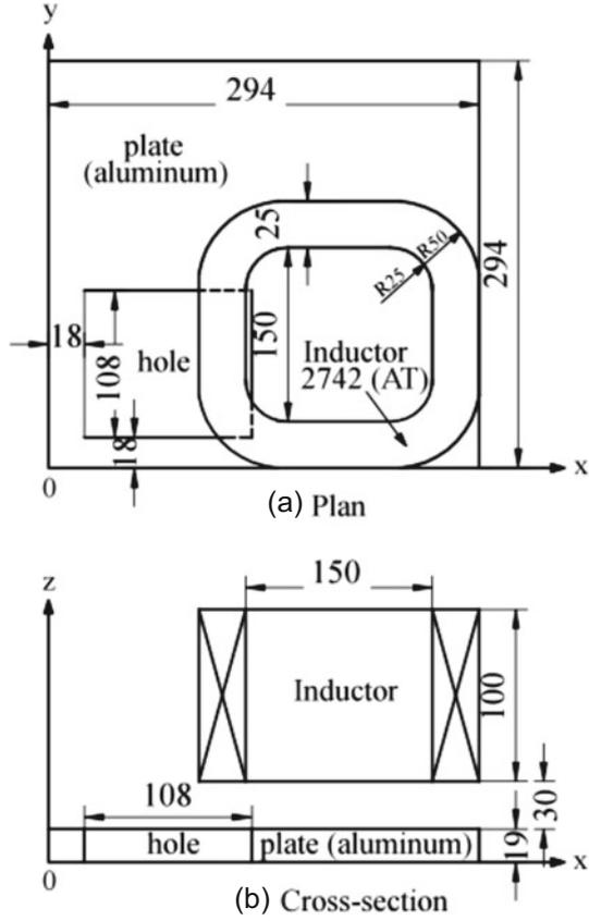
**Fig. 4.** Geometry of TEAM problem 7: inductor and conducting plate with a hole (all dimensions are in mm).
