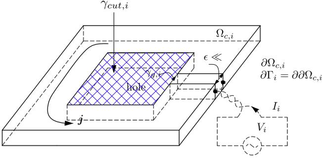
**Fig. 1.** 3D plate with a hole, its associated cut and source of electromotive force.
