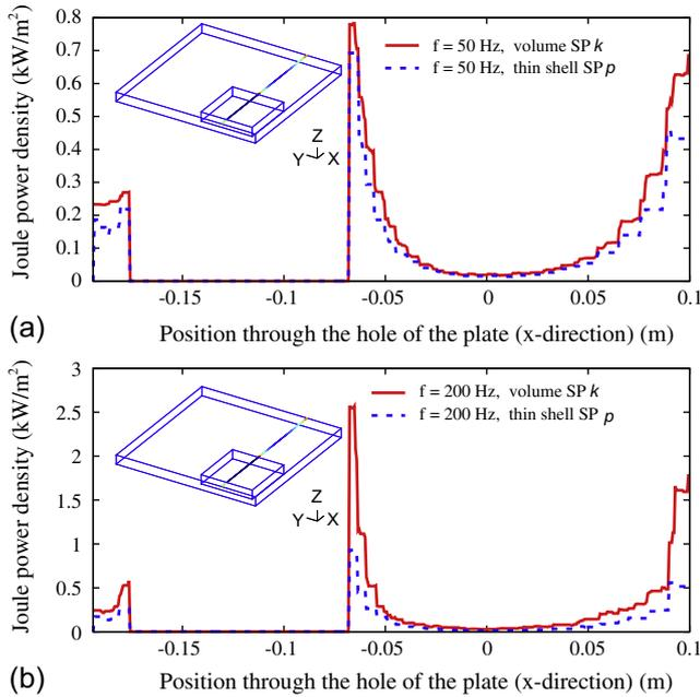
**Fig. 7.** Joule power loss density with TS model and volume correction through the hole ( $d = 19$  mm).
