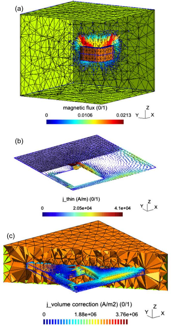
**Fig. 5.** TEAM problem 7: magnetic flux density  $b_u$  (in a cut plane) generated by a stranded inductor (a), TS eddy current density  $\mathbf{j}_p$  (b) and its volume correction (locally focussing on the mesh of plate and its neighborhood)  $\mathbf{j}_k$  (c) ( $d = 19$  mm,  $f = 200$  Hz).
