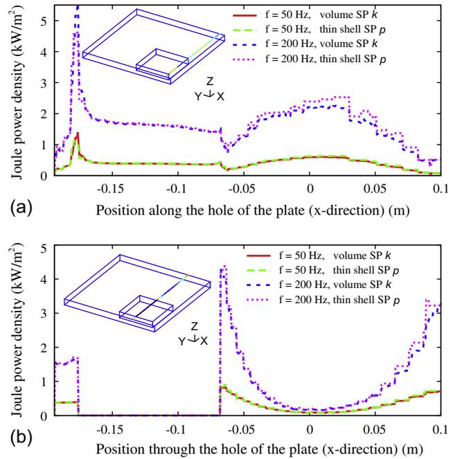
**Fig. 9.** Joule power loss density with TS model and volume correction along hole and plate borders (a), and through the hole (b) ( $d = 2$  mm).
