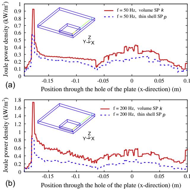
**Fig. 6.** Joule power loss density with TS model and volume correction along hole and plate borders (along the line drawn in the plate geometry) ( $d = 19$  mm).
