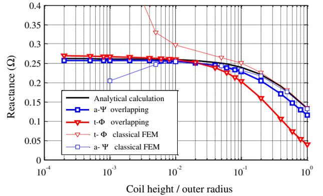
**Fig. 5.** Reactance of the coil vs. height/radius ratio.
