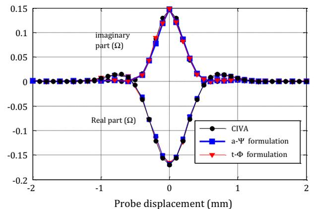
**Fig. 8.** Variation of the probe transimpedance due to the flaw.
