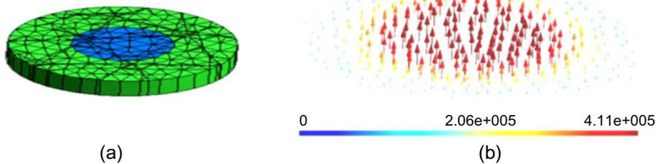
**Fig. 4.** (a) Prismatic mesh of the coil, (b) source vector  $t_0$  (A/m) calculated in each prism of the coil mesh.
