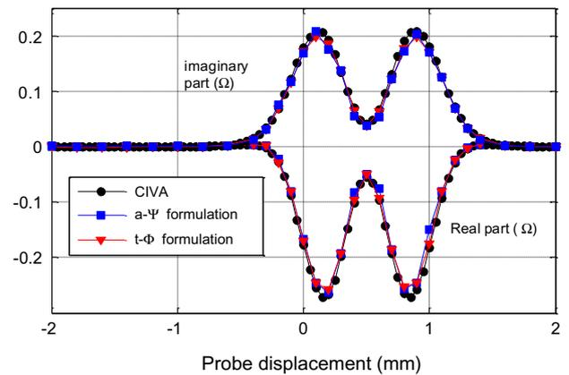
**Fig. 7.** Variation of the transmitter impedance due to the flaw.
