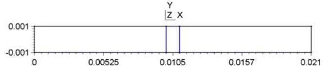
Fig. 3. Geometry of our simulation: Homogeneous wall of thickness  $e = 1 \text{ mm}$  placed in vacuum.
