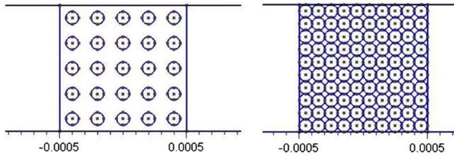
**Fig. 5.** Wall of thickness  $e = 1$  mm partially filled with inclusions of radius  $r_i = 0.05$  mm: (left)  $\tau = 20\%$  (right)  $\tau = 76\%$ .
