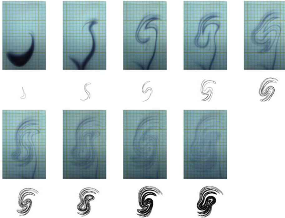
**Fig. 4.** Sequence of blob of dye shape at times  $0, 1/f, \dots, 9/f$ . Experiment (up) and computation (down).
