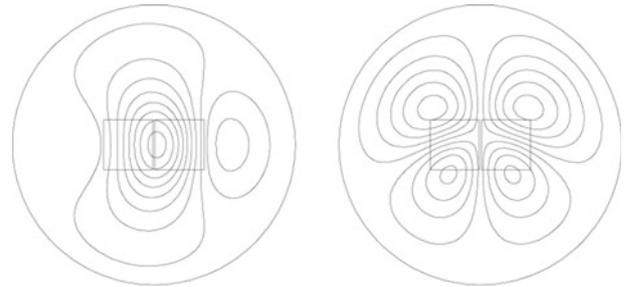
**Fig. 3.** Streamlines of the 2-D velocity field  $\mathbf{v}_u$  on  $\Gamma_t$  for the configurations where the current lines are (almost) horizontal (left) and vertical (right).
