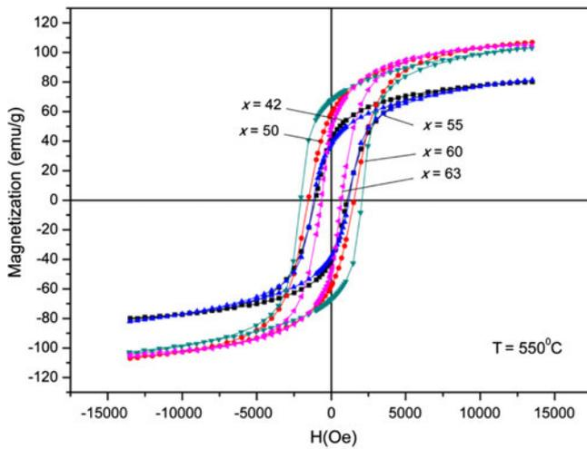
Fig. 4. Room temperature magnetization curves of  $\text{Fe}_x\text{Pd}_{100-x}$  nanoparticles annealed at  $550^\circ\text{C}$  with various  $x$ .
