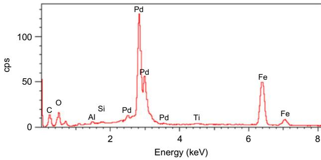
Fig. 3. EDS result of  $\text{Fe}_x\text{Pd}_{100-x}$  nanoparticles with  $x = 60$ .
