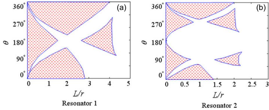
**Fig. 4.** Stability maps of resonators 1 (a) and 2 (b) (with the identical incident angles for all the four mirrors) versus  $L/r$  and  $\theta$ .
