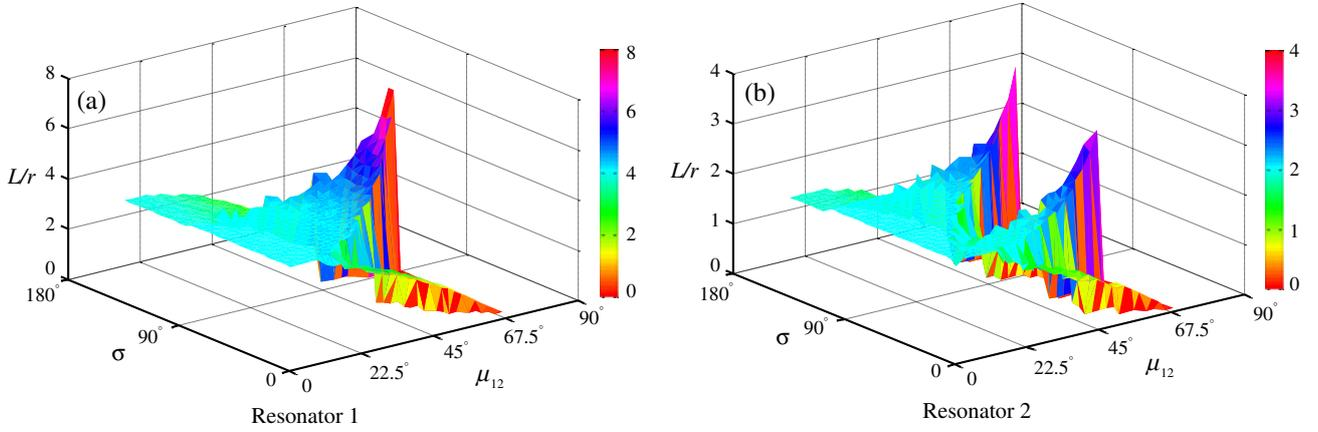
**Fig. 3.** Stability in three dimensions of resonators 1 (a) and 2 (b) versus  $L/r$ , incident angle  $\mu$  and the folding angle  $\sigma$ .
