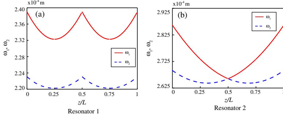
**Fig. 2.** Beam size of the cross section versus the propagation distance in resonators 1 (a) and 2 (b).
