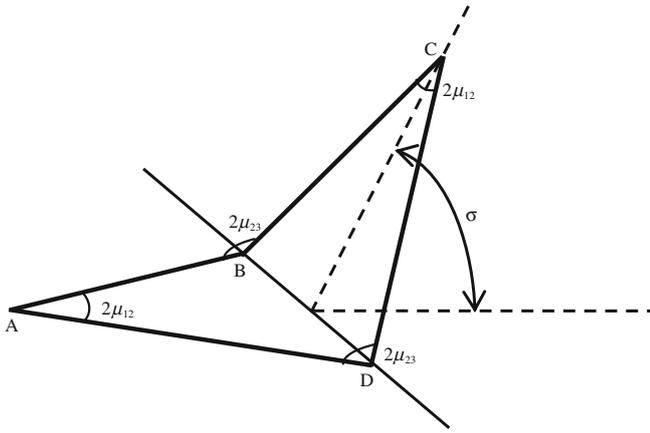
**Fig. 1.** Geometrical construction of a nonplanar ring resonator.
