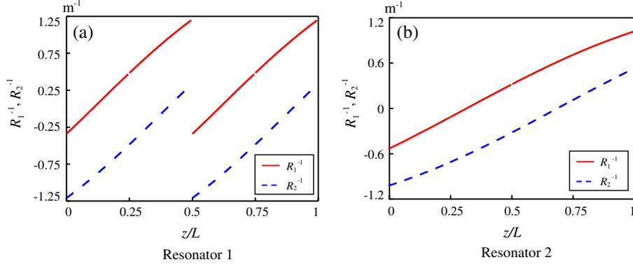
**Fig. 6.** Wave-front radii of curvature  $R_1^{-1}$  and  $R_2^{-1}$  of the laser beam versus the propagation distance in resonators 1 (a) and 2 (b).
