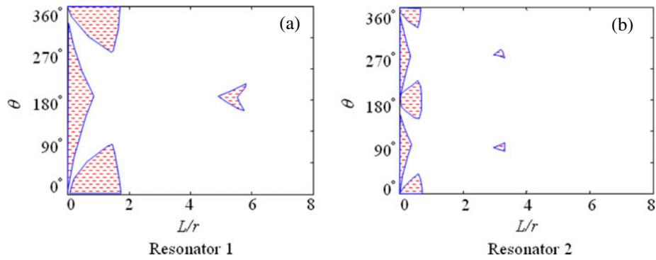
**Fig. 5.** Stability maps of resonators 1 (a) and 2 (b) (when the incident angles are unequal for the mirrors) versus the image rotation angle  $\theta$  and  $L/r$ . The incident angles on mirror A are  $65^\circ$  and  $70^\circ$  in resonators 1 and 2, respectively.
