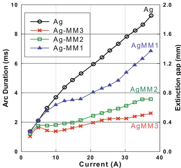
Fig. 8. (Color online) Arc duration versus Current for Ag, AgMM1, AgMM2 and AgMM3 at 20 cm/s 42 VDC resistive.
