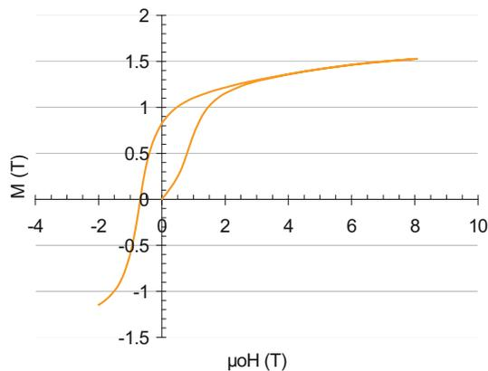
**Fig. 4.** (Color online)  $M = f(\mu_0 H)$  for magnetic phase in electrical contact material.
