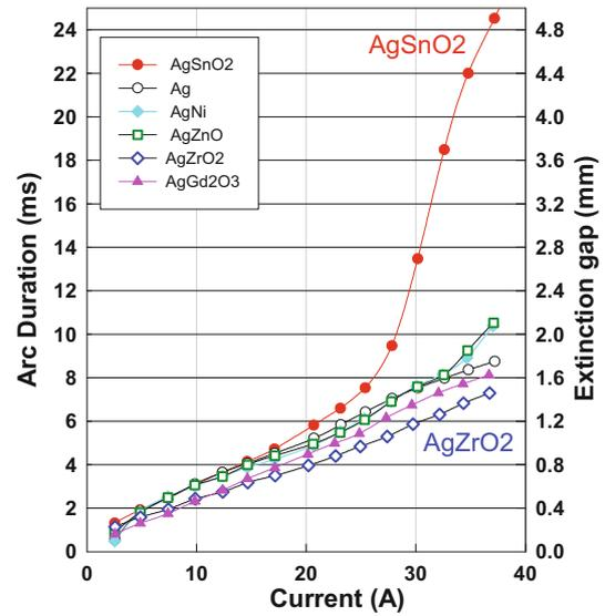
Fig. 2. (Color online) 42 VDC resistive,  $t = f(I)$ , Ag, AgNi, AgSnO<sub>2</sub>, AgZnO, AgGd<sub>2</sub>O<sub>3</sub>, AgZrO<sub>2</sub>.
