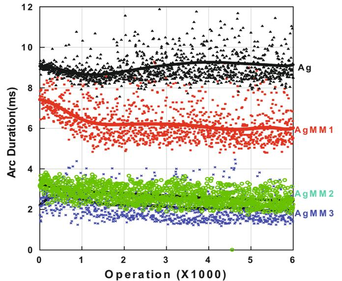
Fig. 10. (Color online) Arc duration versus number of break operations for Ag, AgMM1, AgMM2 and AgMM3 at 20 cm/s 42 VDC, 37.5 A at 20 cm/s.
