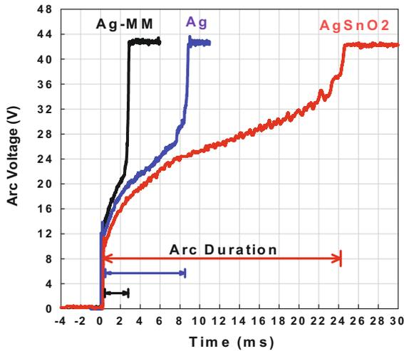
Fig. 7. (Color online) Arc voltage versus time for AgSnO<sub>2</sub>, Ag and AgMM3 at 42 VDC, 37.5 A resistive.
