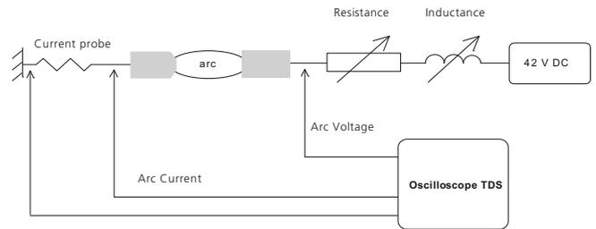
**Fig. 5.** Electrical test apparatus for break arc.
