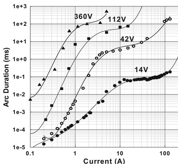
**Fig. 1.** Arc duration versus current in a range from 0.1 to up to 100 A at four circuit voltage (14, 42, 112 and 360 VDC).
