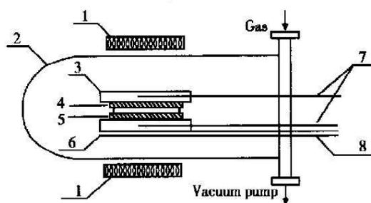
**Fig. 1.** Schematic of apparatus of CSS 1: Halogen tungsten lamp, 2: Quartz tube, 3: Upper graphite block, 4: Substrate, 5: CdTe source, 6: Lower graphite block, 7: Thermocouple, 8: Holding rod.
