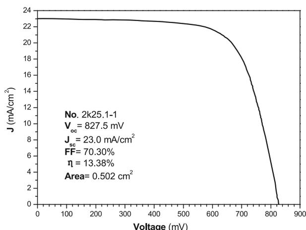
Fig. 4.  $I - V$  curver of  $0.501 \text{ cm}^2$  CdS/CdTe/ZnTe:Cu thin film solar cell.
