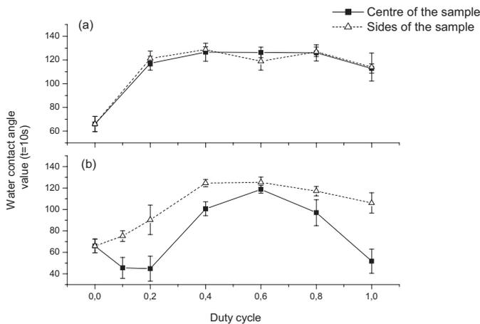
**Fig. 5.** Water contact angle value 10 s after the deposit of the drop as a function of the duty cycle on the centre and on the sides of the sample ( $d = 1.8$  cm,  $P = 900$  W,  $Q = 40$  SL/min,  $E = 16.2$  kJ (a) and  $E = 56.7$  kJ (b)).
