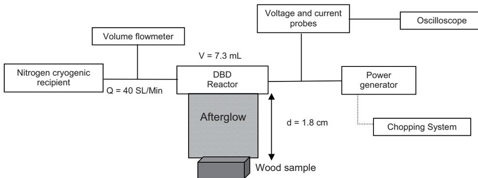
Fig. 1. Scheme of the experimental set-up.
