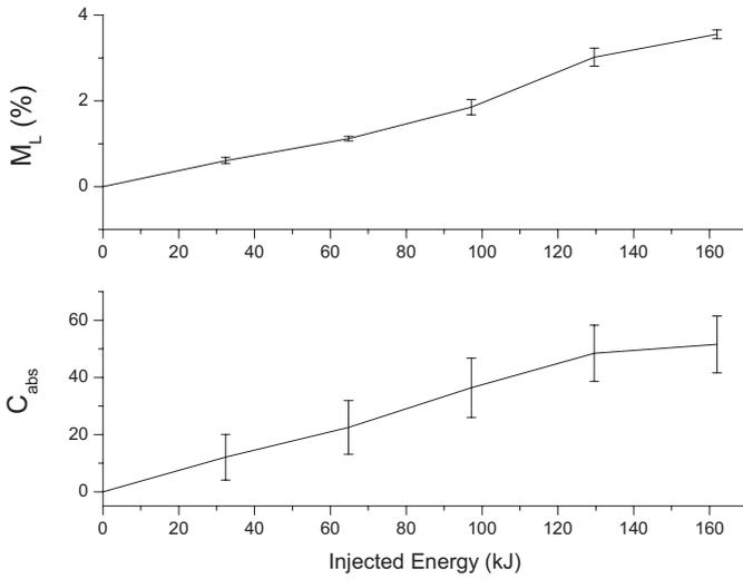
**Fig. 3.** Mass loss during treatment ( $M_L$ ) and absorption parameter ( $C_{abs}$ ) as a function of injected energy ( $d = 1.8$  cm,  $P = 900$  W,  $r_c = 1$ ,  $Q = 40$  SL/min).
