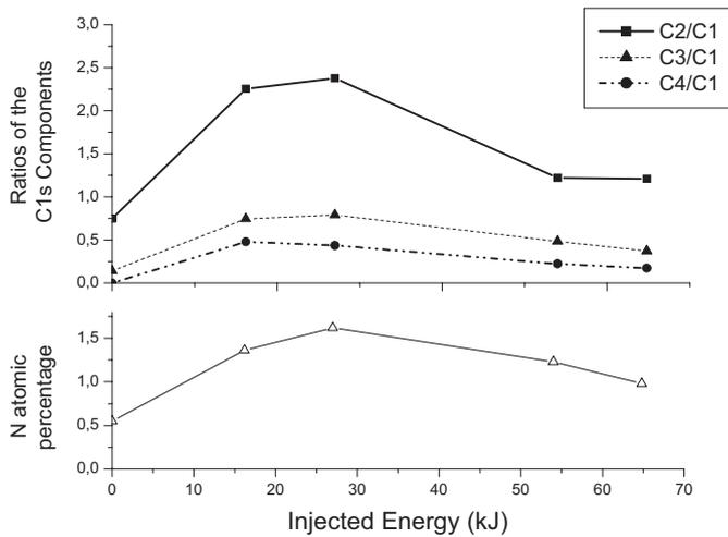
**Fig. 6.** Evolution of the  $C_2/C_1$ ,  $C_3/C_1$  and  $C_4/C_1$  ratios and Nitrogen atomic percentage as a function of the injected energy ( $d = 1.8$  cm,  $P = 900$  W,  $r_c = 1$ ,  $Q = 40$  SL/min).
