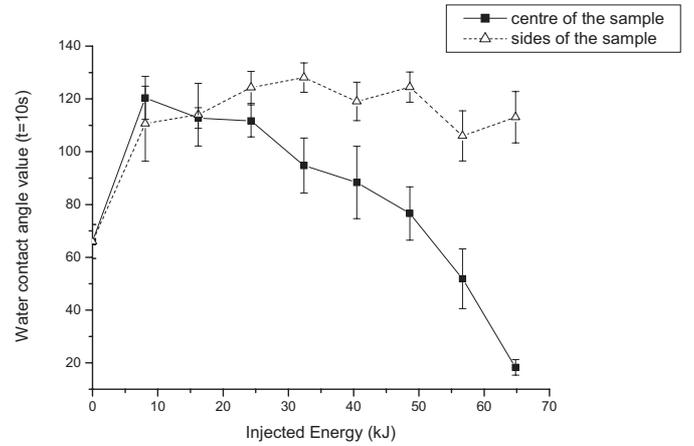
**Fig. 4.** Water contact angle value 10 s after the deposit of the drop as a function of injected energy on the centre and on the sides of the sample ( $d = 1.8$  cm,  $P = 900$  W,  $r_c = 1$ ,  $Q = 40$  SL/min).
