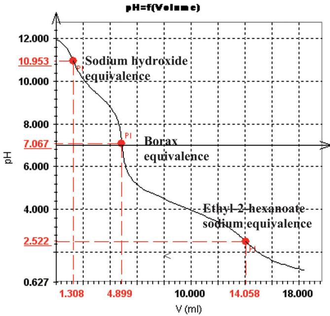
Fig. 2. Characteristic curve obtained by acid-base titration of fungicide solutions.
