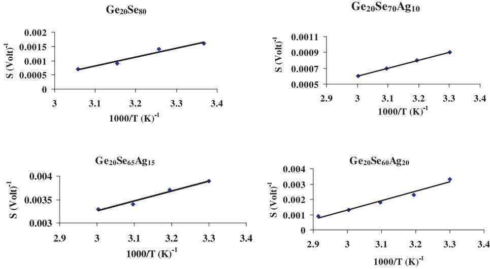
Fig. 3. Slope ( $S$ ) vs.  $1000/T$  curves for a- $\text{Ge}_{20}\text{Se}_{80-x}\text{Ag}_x$  system.
