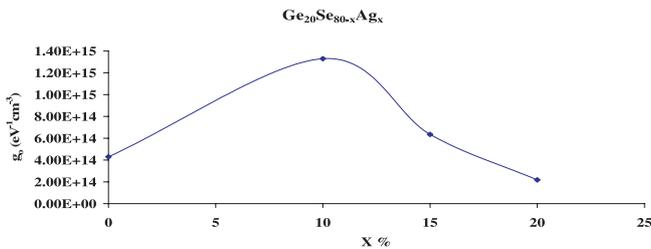
**Fig. 5.** Density of localized states ( $g_0$ ) vs. Ag concentration in a-Ge<sub>20</sub>Se<sub>80-x</sub>Ag<sub>x</sub> system.
