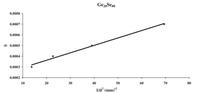
Fig. 4. Slope ( $S$ ) vs.  $1/d^2$  curve for  $\text{Ge}_{20}\text{Se}_{80}$  alloy at a fixed temperature 301 K.
