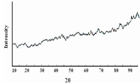
Fig. 1. X-ray diffraction pattern for  $\text{Ge}_{20}\text{Se}_{70}\text{Ag}_{10}$  alloy.
