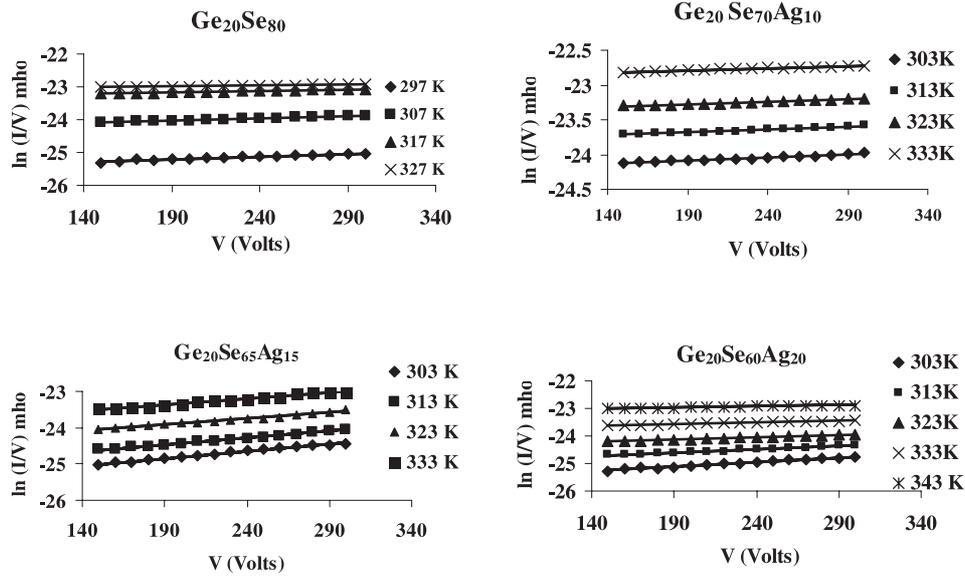
Fig. 2.  $\ln I/V$  vs.  $V$  curves at different temperatures for a- $\text{Ge}_{20}\text{Se}_{80-x}\text{Ag}_x$  system.
