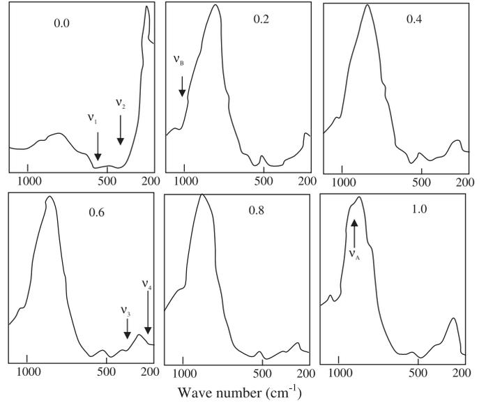
**Fig. 6.** The recorded infrared spectra of the ferrites  $\text{Mn}_{0.5}\text{Zn}_{0.5}\text{Al}_x\text{Fe}_{2-x}\text{O}_4$ .
