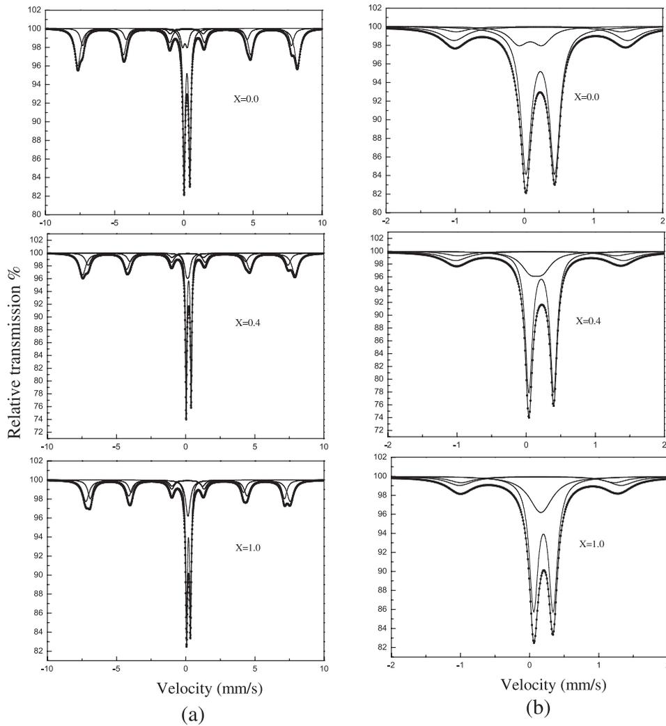
**Fig. 1.** (a) Some of the similar Mössbauer spectra of the  $\text{Mn}_{0.5}\text{Zn}_{0.5}\text{Al}_x\text{Fe}_{2-x}\text{O}_4$  ferrites taken at room temperature for  $x = 0, 0.4$  and  $1$ , and (b) their corresponding central paramagnetic phase.
