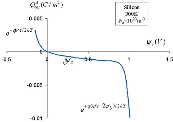
Fig. 1.  $Q\Psi$  graph: SC charge per unit area versus surface potential.
