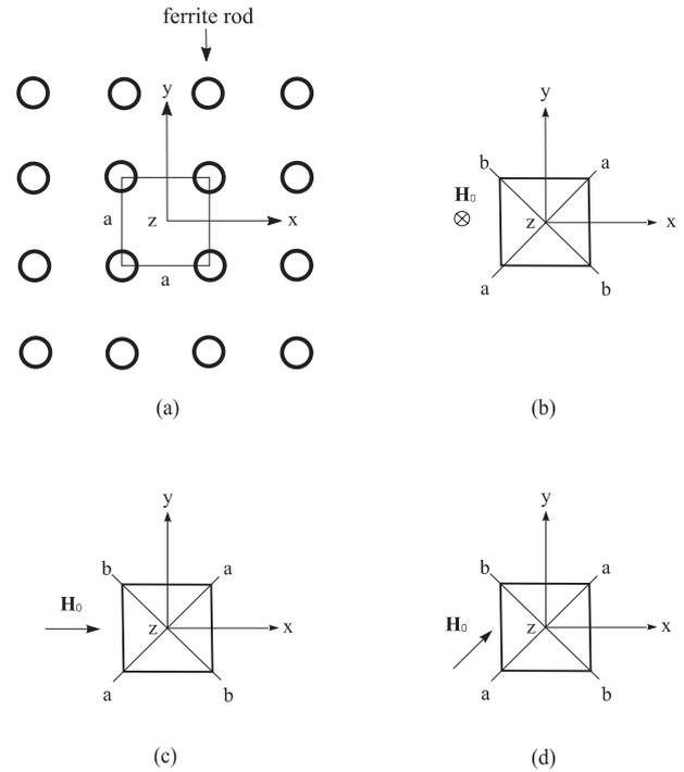
**Fig. 1.** (a) 2D square lattice of circular cross-section ferrite rods, (b) the unit cell magnetized by  $\mathbf{H}_0 \parallel z$ , (c) the unit cell magnetized by  $\mathbf{H}_0 \parallel x$ , (d) the unit cell magnetized by  $\mathbf{H}_0 \parallel (a - a)$ .
