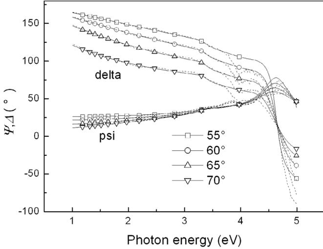
**Fig. 3.** Measured  $\Psi$  and  $\Delta$  (dash lines) and the one-oscillator LOM fit (solid lines) for VASE at the energy range from 1.0 to 5.0 eV.
