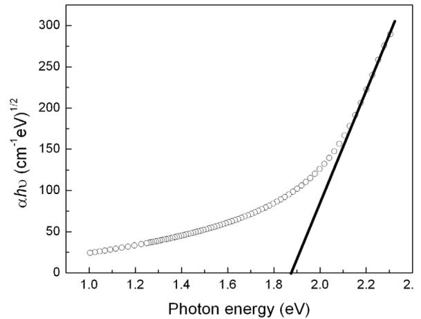
**Fig. 6.** Fitting of the absorption edge data to the amorphous semiconductors model.
