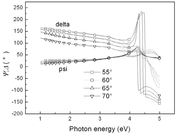
**Fig. 2.** Measured  $\Psi$  and  $\Delta$  (dash lines) and the Cauchy model fit (solid lines) for VASE at the energy range from 1.0 to 5.0 eV.
