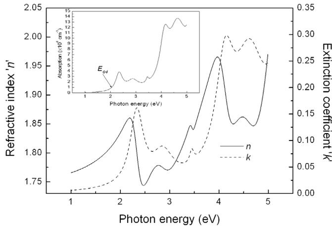
**Fig. 5.** Refractive index and extinction coefficient of NPAMLI obtained by six-oscillator LOM fit. Inset is the absorption spectra calculated from extinction coefficient.
