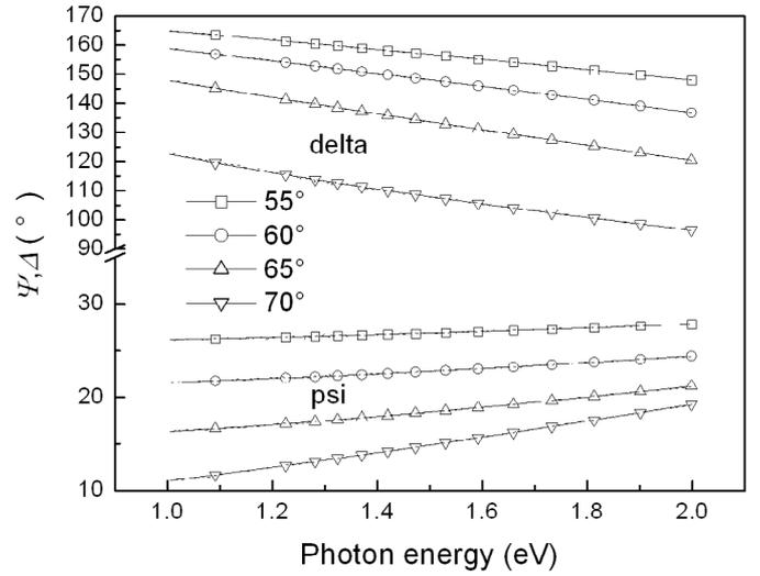
**Fig. 1.** Measured  $\Psi$  and  $\Delta$  (dash lines) and the Cauchy model fit (solid lines) for VASE at the energy range from 1.0 to 2.0 eV.
