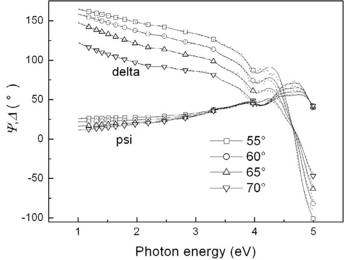
**Fig. 4.** Measured  $\Psi$  and  $\Delta$  (dash lines) and the six-oscillator LOM fit (solid lines) for VASE at the energy range from 1.0 to 5.0 eV.
