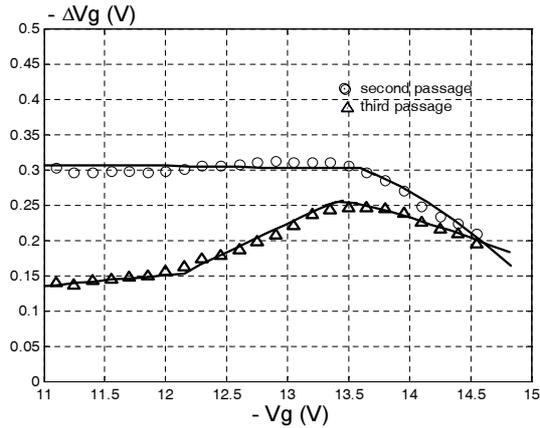
**Fig. 9.** Modelling of experimental  $\Delta Vg(Vg)$  characteristics of Figure 8A.
