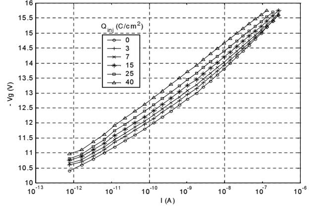
**Fig. 6.** Typical influence of constant current injection corresponding to that of Figure 5 on  $I(Vg)$  characteristic ( $Vg < 0$ ) obtained after removing the excess current at low field [1,13].
