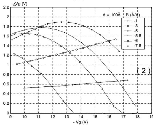
**Fig. 2.** Typical centroid calculated displacement influence of a negative charge of density  $5 \times 10^{12} \text{ cm}^{-2}$  on the  $\Delta Vg(Vg)$  characteristics (see insert figure).  $\phi_m = 3 \text{ eV}$ ,  $D_{ox} = 110 \text{ \AA}$ .
