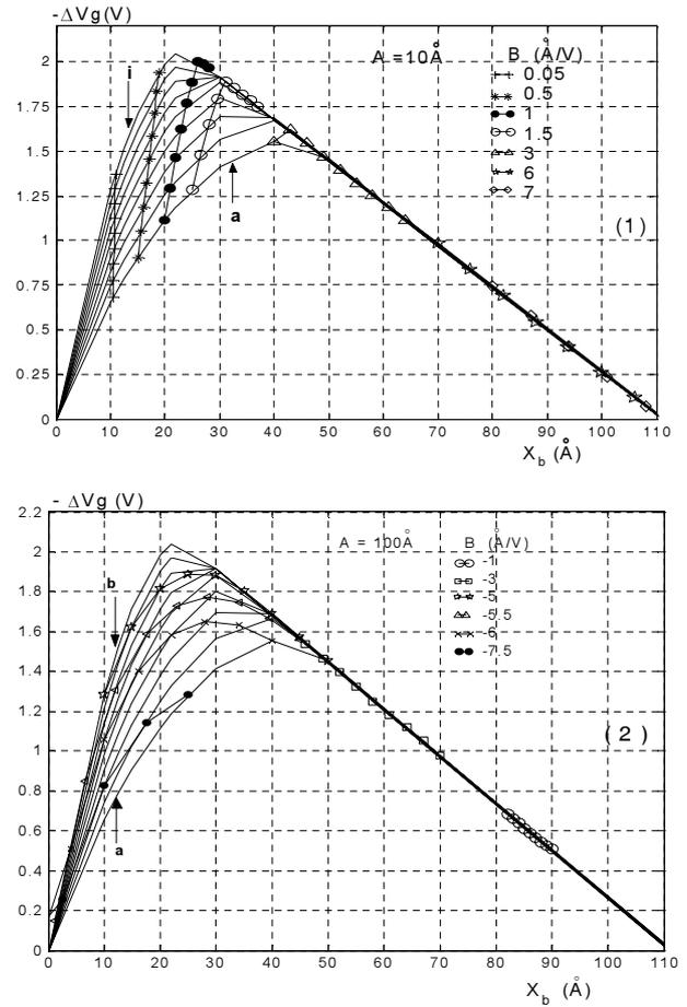
**Fig. 3.** Typical calculated influence of the centroid of a negative charge of density  $5 \times 10^{12} \text{ cm}^{-2}$  on the  $\Delta Vg$  shift with respect to the voltage ( $Vg$ ).  $\phi_m = 3 \text{ eV}$ ,  $D_{ox} = 110 \text{ \AA}$ .
