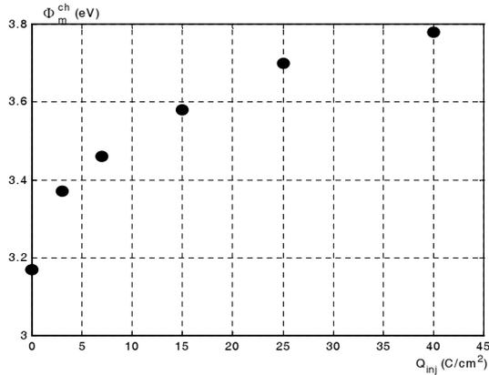
**Fig. 10.** Injected charge influence on the effective barrier determined from FN plot at high field ( $-Vg > 13.5$  V).  $D_{ox} = 109$  Å,  $S = 10^{-6}$  cm<sup>2</sup>,  $I = 10^{-8}$  A.
