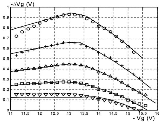
**Fig. 7.** Typical  $\Delta Vg(Vg)$  characteristics obtained from Figure 6 after each current injection. experiment:  $Q_{inj}$  ( $C/cm^2$ ): ( $\nabla$ ) 3, ( $\square$ ) 7, ( $\triangle$ ) 15, ( $+$ ) 25, ( $\circ$ ) 40. (—) theory:
