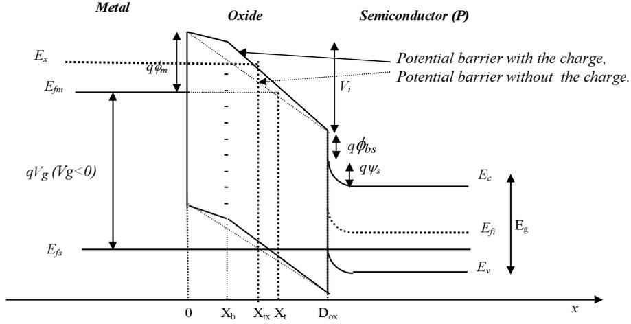
**Fig. 1.** Energy band diagram of MOS structures with and without of the negative charge of density  $N_1$  situated at  $x = X_b$  in the oxide for a given voltage  $Vg$ , where
