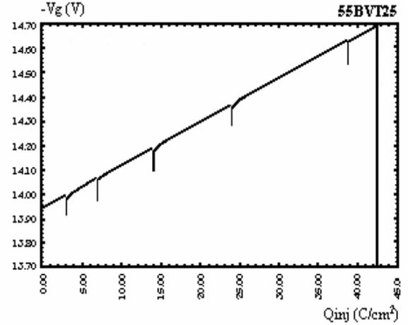
**Fig. 5.** Typical  $Vg(Q_{inj})$  characteristic sequences obtained after current injection to breakdown,  $D_{ox} = 109 \text{ \AA}$ ,  $S = 10^{-6} \text{ cm}^2$ ,  $I = 10^{-8} \text{ A}$ .
