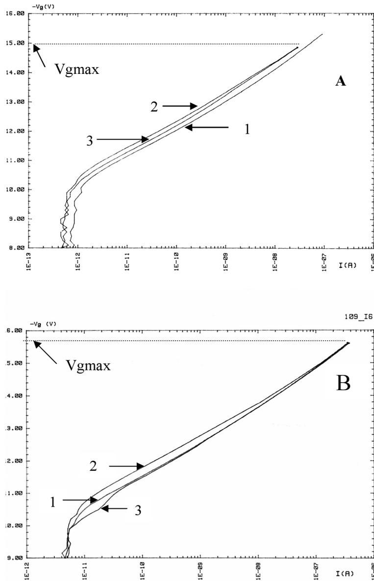
**Fig. 8.** Typical influence of the voltage ( $V_{gmax}$ ), fixed by the second  $I(Vg)$  characteristic on the third one.  $D_{ox} = 109 \text{ \AA}$ ,  $S = 10^{-6} \text{ cm}^2$ ,  $I = 10^{-8} \text{ A}$ .  $V_{gmax}$  (V): (A)  $-15$ , (B)  $-15.7$ . (1)  $I(Vg)$  first passage (before injection), (2)  $I(Vg)$  second passage (after injection), (3)  $I(Vg)$  third passage.
