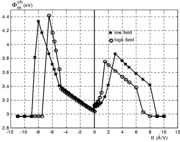
**Fig. 4.** Centroid movement influence of a negative charge of density  $5 \times 10^{12} \text{ cm}^{-2}$  on the apparent barrier ( $\Phi_m^{ch}$ ) at low and high field.  $\phi_m = 3 \text{ eV}$ ,  $D_{ox} = 110 \text{ \AA}$ .
