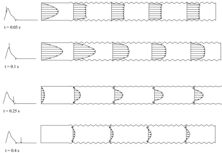
**Fig. 6.** Evolution of axial velocity profiles during the cardiac pulse.
