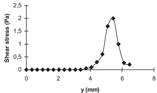
**Fig. 8.** Shear stress distribution near the prosthesis wall at  $t = 0.1$  s.
