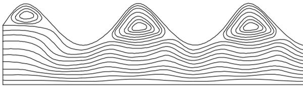
**Fig. 7.** Streamlines contours near crimping at  $t = 0.1$  s.
