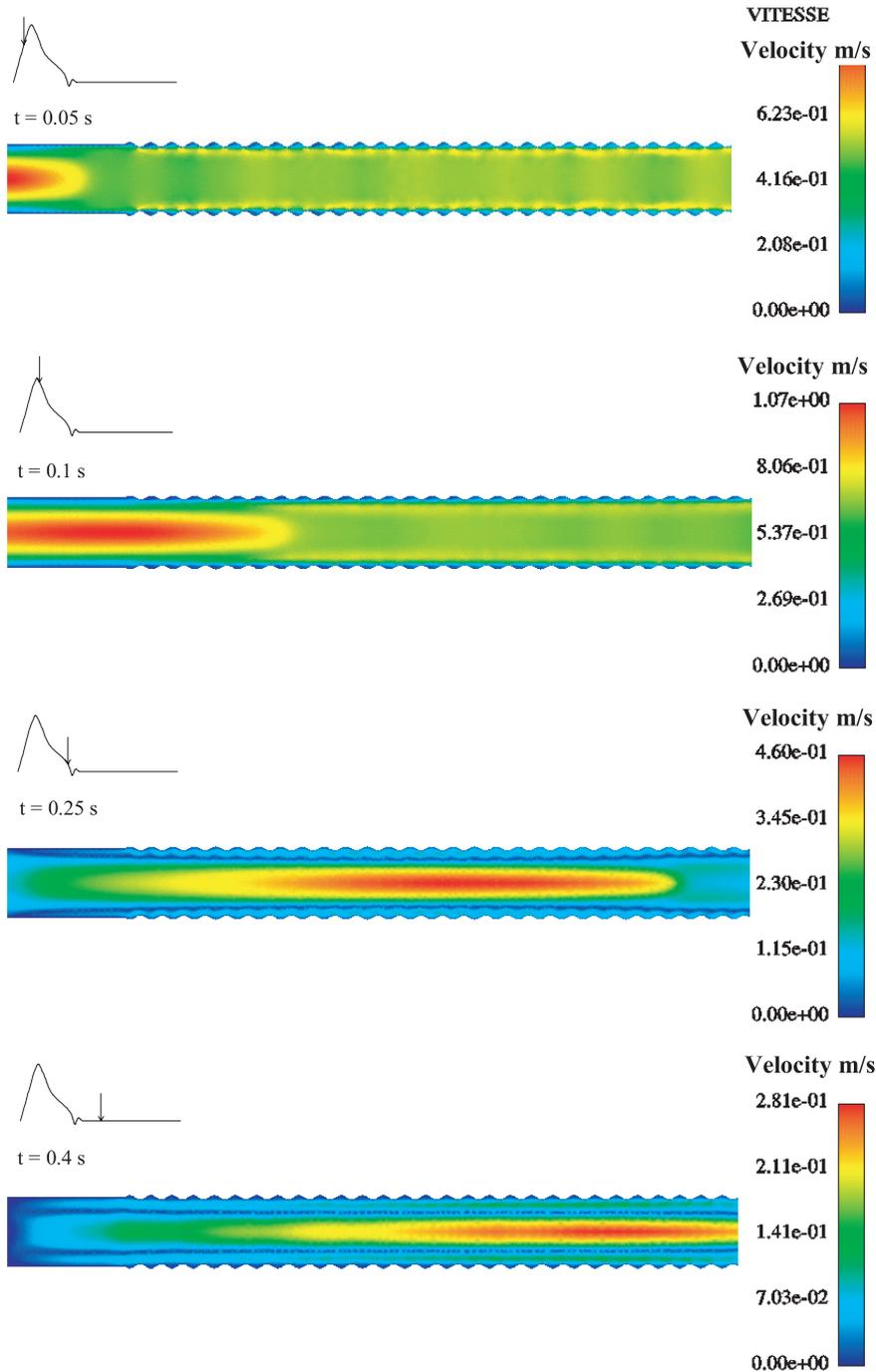
**Fig. 5.** Evolution of isovelocity cartography during the cardiac pulse.
