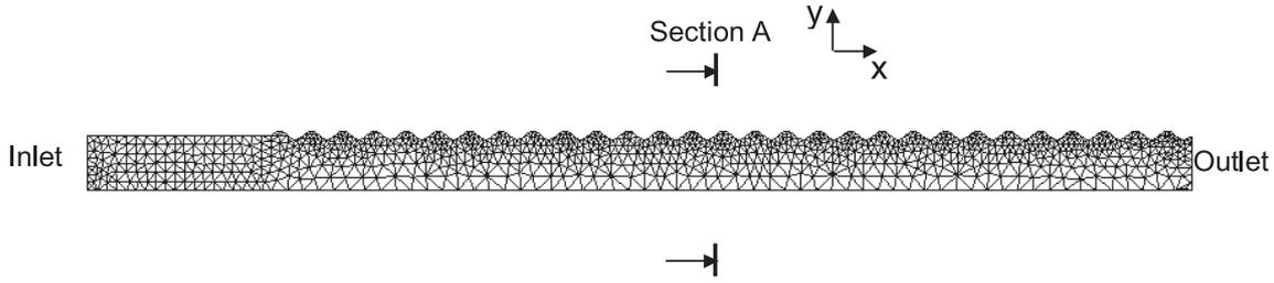
**Fig. 3.** Typical axisymmetric mesh for pulsatile computations.
