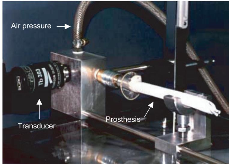
Fig. 2. Prosthesis deformation device.
