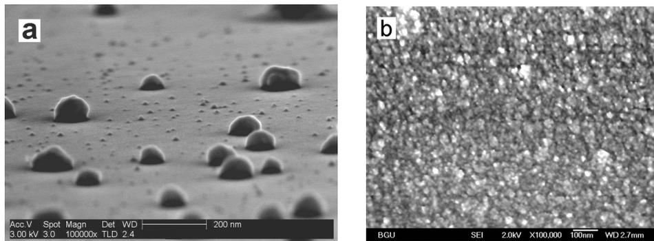
**Fig. 4.** (a) FEG-SEM images of chemically deposited PbSe films deposited on Si(100) substrates. (b) GaAs(100) substrates.
