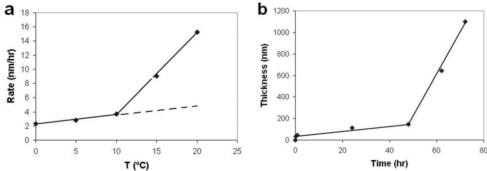
**Fig. 2.** (a) Film growth rate plotted vs. deposition temperature. (b) Film thickness plotted vs. deposition time for constant deposition temperature of 20 °C.
