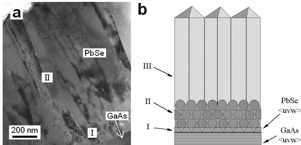
**Fig. 1.** (a) TEM cross-section of PbSe on GaAs showing the two distinct regions present in the film. (b) Schematic illustration showing the morphology evolution in PbSe films on GaAs as a function of thickness. The  $\langle u,v,w \rangle$  indices denote the substrate orientation and the corresponding direction of the PbSe film growth.
