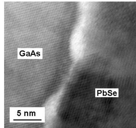
**Fig. 3.** HRTEM cross-sectional image showing an area in which direct contact between GaAs(100) and PbSe is observed.
