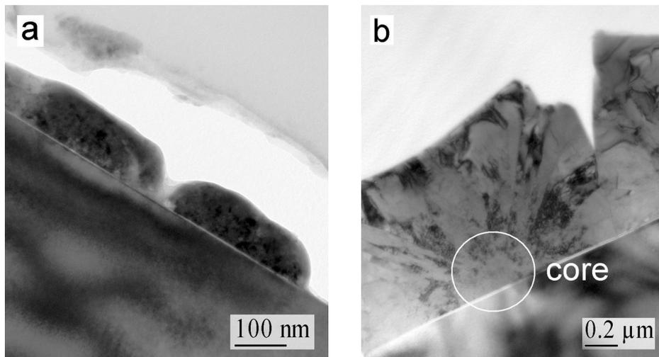
**Fig. 5.** (a) TEM cross-sectional images showing PbSe deposited on Si(100) at a deposition temperature of 0 °C. (b) 20 °C.
