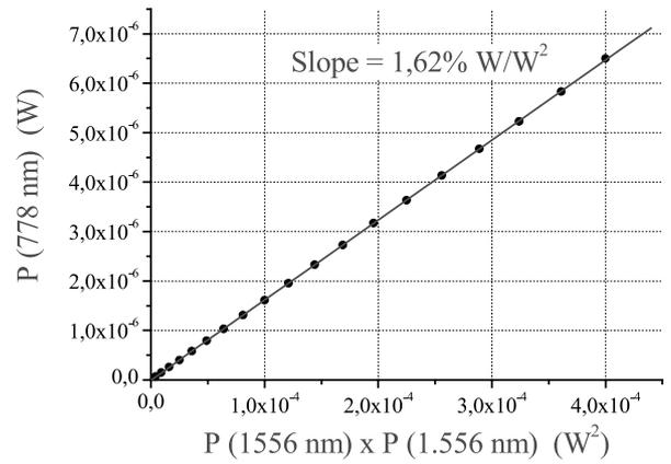
**Fig. 3.** Variation of the SH power at 778 nm *versus* the fundamental power square at 1556 nm.
