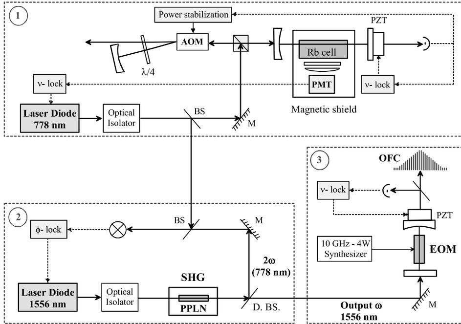
**Fig. 1.** Diagram of the experimental set-up. Part 1: Rb optical frequency standard set-up; Part 2: SHG in a PPLN crystal; Part 3: OFC based on the use of an EOM placed inside a Fabry-Perot cavity. AOM: Acousto-Optic Modulator; PMT: Photomultiplier Tube; PZT: Piezoelectric transducer; BS: Beamsplitter; D. BS: Dichromatic Beamsplitter; M: Mirror;  $\nu$ -lock: frequency lock;  $\phi$ -lock: phase lock.
