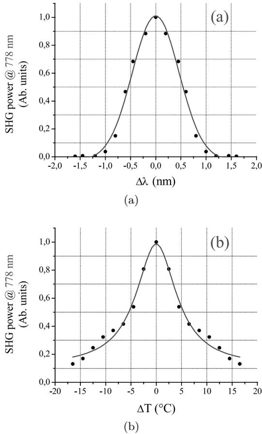
**Fig. 4.** Wavelength and temperature acceptances.
