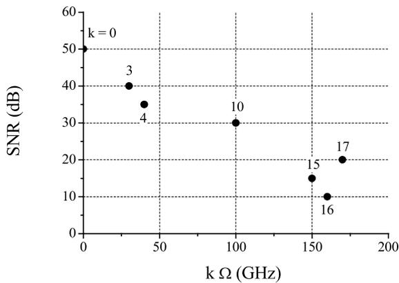
**Fig. 6.** SNR of the beatnotes between the OFC and the tuneable auxiliary laser diode around 1556 nm.
