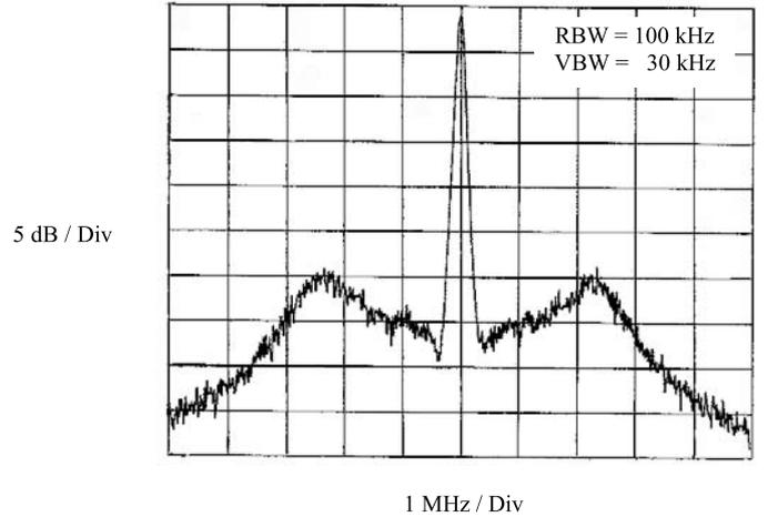
**Fig. 5.** Beatnote between the Rb optical frequency standard at 778 nm and the frequency doubled 1556 nm ECLD.
