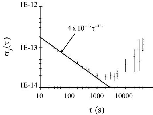
**Fig. 2.** Allan standard deviation of the beatnote between two similar and independent Rb optical frequency standard at 778 nm.
