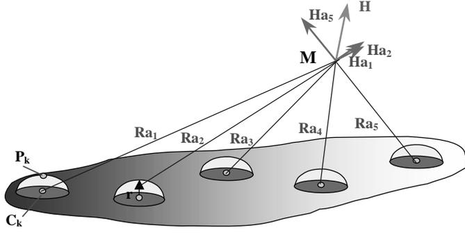
Fig. 1. Discretization of the core surface into a finite number of hemispherical sources.
