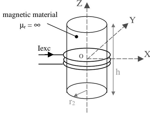
Fig. 2. Geometry under test.
