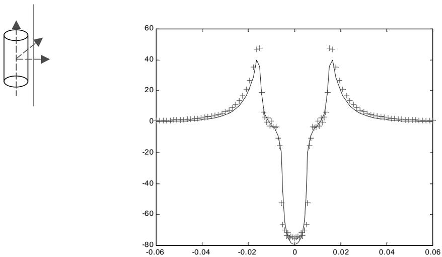
**Fig. 7.**  $H_z$  component of the induction field  $H$  as a function of height  $z$  (position 2).
