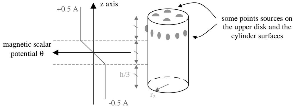
Fig. 3. Magnetic scalar potential boundary conditions.
