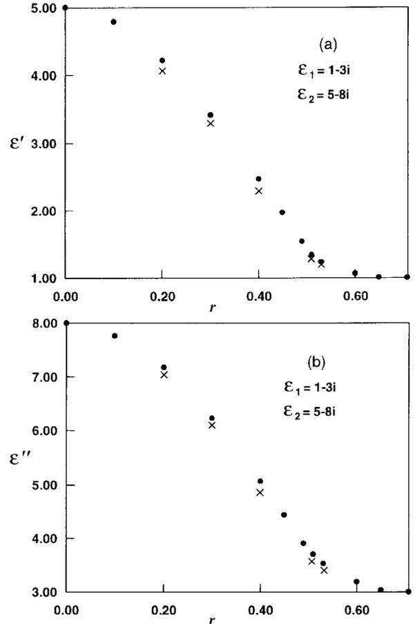
**Fig. 8.** (a) Comparison of the real part of the complex effective dielectric constant evaluated by the finite-element method (●) and the 2-pole Bergman-Milton approximation (×, Ref. [19]) as a function of the radius of the circular cylinder  $r$ . The dielectric constants of the two-component composite material are  $\varepsilon_1 = 1 - 3i$  and  $\varepsilon_2 = 5 - 8i$ . (b) Same as in (a) for the imaginary part of the complex effective dielectric constant.
