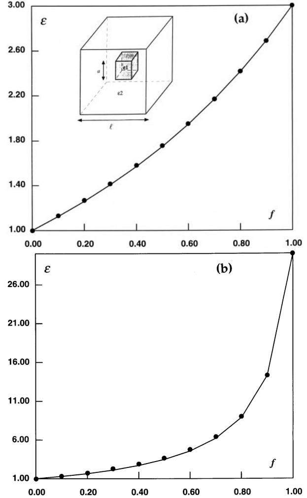
**Fig. 6.** (a) The effective permittivity (solid circle) is shown as a function of the volume fraction  $f$  of the inclusion phase. Cubic inclusions (permittivity  $\epsilon_1 = 3$ ) are placed in a host matrix material of permittivity  $\epsilon_2 = 1$ . The inset shows the configuration studied. Simple cubic lattice. The solid line shown in this figure corresponds to results obtained from Maxwell Garnett equation. (b) Same as in (a) for  $\epsilon_1 = 30$  and  $\epsilon_2 = 1$ .
