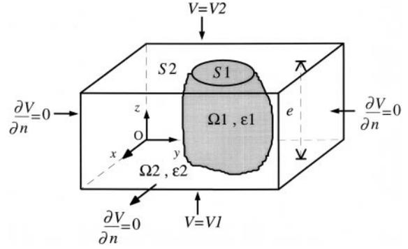
**Fig. 2.** Same as in Figure 1 for a fused inclusion with dielectric constant  $\varepsilon_1$ . This configuration corresponds to high concentrations of inclusions.
