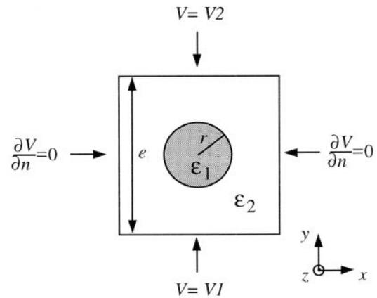
**Fig. 7.** Unit cell of a simple square lattice of identical discoidal inclusions with permittivity  $\epsilon_1$  embedded in a host material with permittivity  $\epsilon_2$ .
