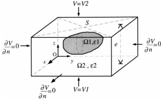
**Fig. 1.** A schematic diagram of the unit cell of the two-component periodic composite (three-dimensional) material investigated in the numerical computation. The isolated inclusion with dielectric constant  $\varepsilon_1$  is periodically arranged in a three-dimensional structure. The dielectric constant of the remaining space is  $\varepsilon_2$ . See text for notations. This configuration corresponds to low concentrations of inclusions.
