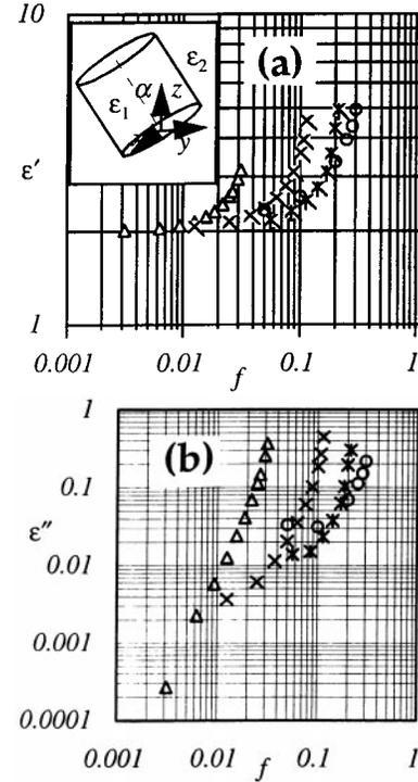
**Fig. 10.** (a) Same as in Figure 9a for the real part of the effective permittivity. The rod axis is oriented at  $30^\circ$  with respect to the electric field vector direction, *i.e.* the  $z$ -direction. (b) Same as in Figure 9b for the imaginary part of the effective permittivity.
