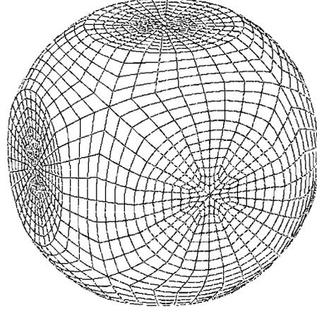
**Fig. 3.** A computational mesh of the spherical inclusion in the unit cell of the composite beyond the touching sphere condition.
