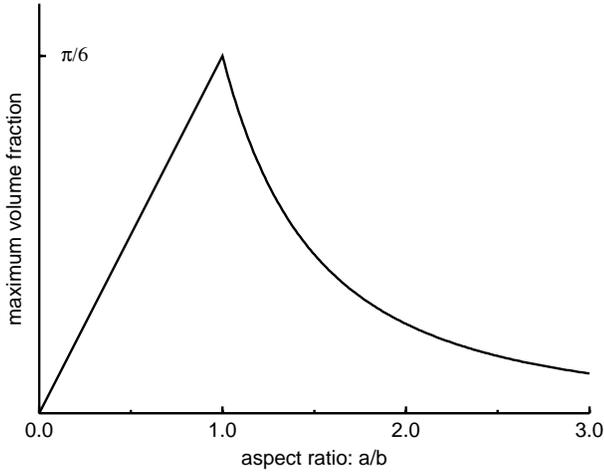
**Fig. 1.** The maximum particle volume fraction,  $f_{\max}$ , as a function of particle aspect ratio,  $\epsilon$ , for a simple-cubic lattice of spheroidal particles with axes of rotation aligned with one of the lattice vectors.
