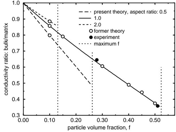
**Fig. 3.** As for Figure 2 but with insulating particles in a highly conducting matrix.
