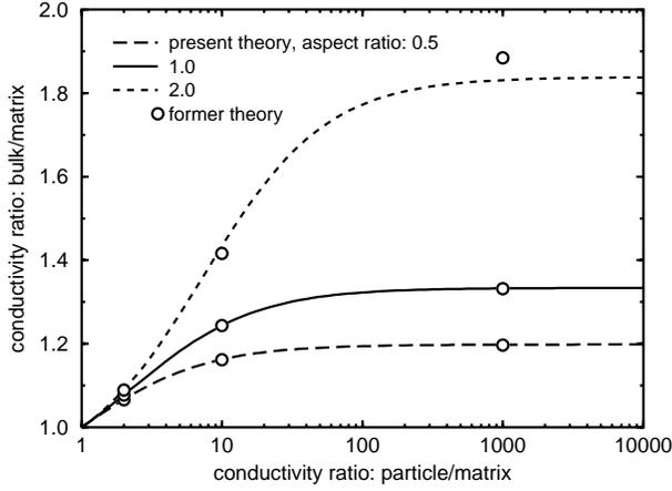
**Fig. 4.** Bulk conductivity as a function of the particle/matrix conductivity ratio  $\alpha$  for  $\alpha \geq 1$  and volume fraction 0.1. The results of former theory are taken from [7].
