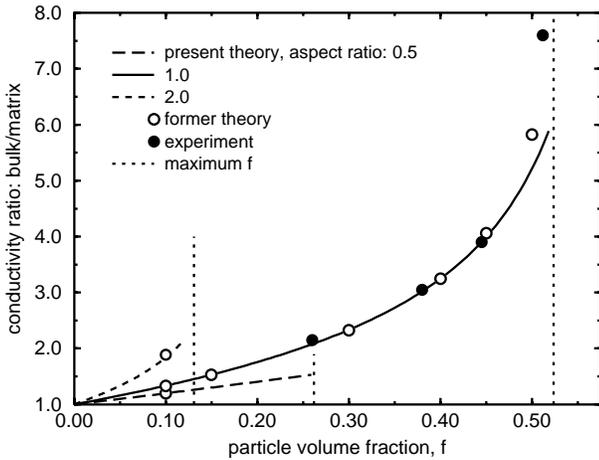
**Fig. 2.** Bulk conductivity as a function of particle volume fraction for highly conducting particles in an insulating matrix. The results of former theory are taken from [7] and the experimental data is taken from [12].
