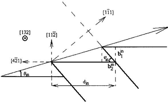
Fig. 10. Intrinsic stacking fault twin mechanism (not drawn at the right scale).
