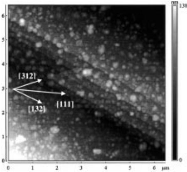
**Fig. 5.** Twinned band fine structure. The scan size is about  $6 \times 6 \mu\text{m}^2$  with a height extension of 138 nm.
