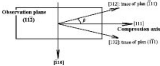
Fig. 1. CuAl specimen configuration.
