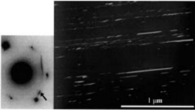
**Fig. 6.** Bright twins in the bulk CuAl single crystal. The spot (111) used for the TEM micrograph in dark field is indicated by an arrow on the diffraction pattern.
