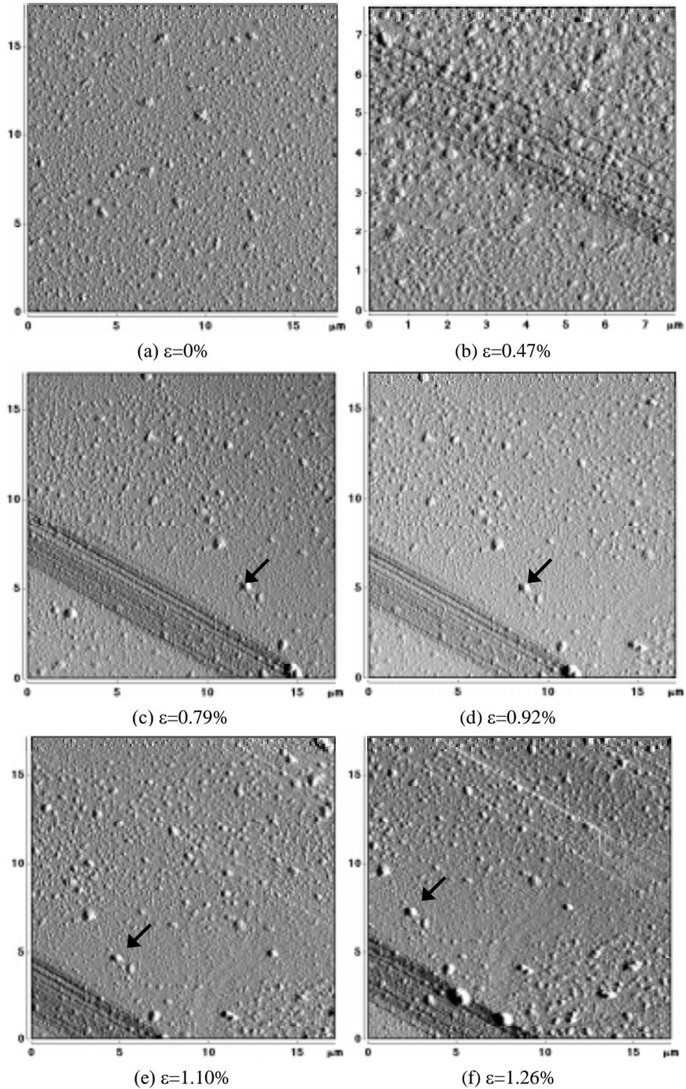
**Fig. 3.** *In situ* deformed CuAl atomic force micrographs. The AFM images presented here have been taken in error signal mode and the scan size is indicated beside.
