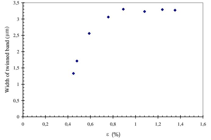
**Fig. 7.** Twinned micro-band width *vs.* specimen strain.
