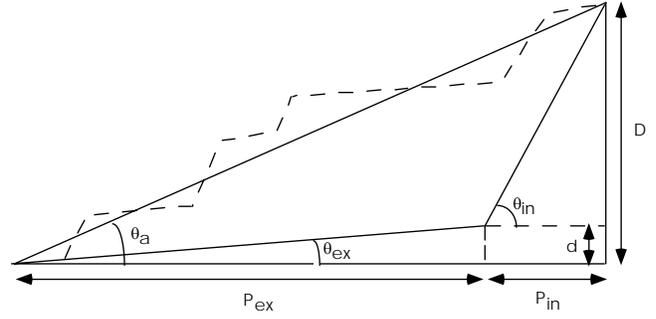
Fig. 11. Schematic representation of the respective contributions  $P_{in}$  and  $P_{ex}$  of each mechanism in twinning.
