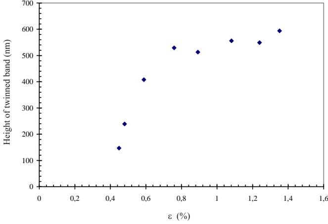
Fig. 8. Twinned micro-band height *vs.* specimen strain.
