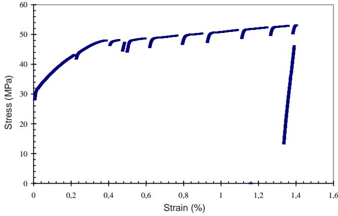
**Fig. 4.** CuAl stress-strain curve. The discontinuities are explained by both the drift of the piezo-actuator and the sample stress relaxation after each stop of the experimental device.
