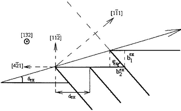
Fig. 9. Extrinsic stacking fault twin mechanism (not drawn at the right scale).
