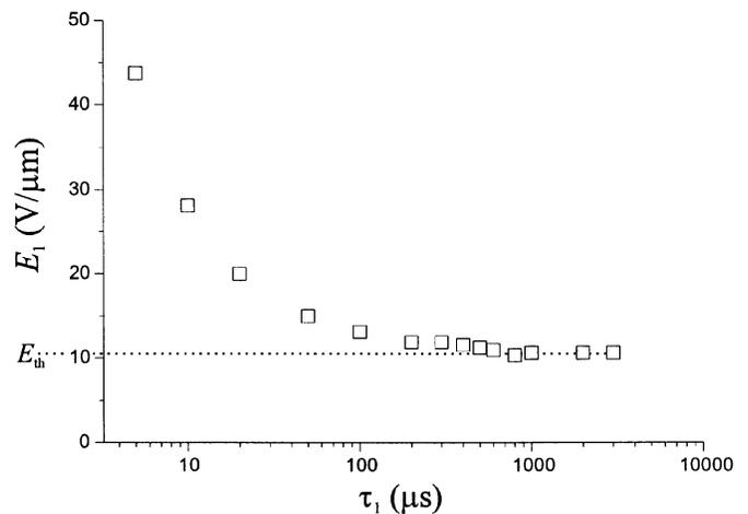
**Fig. 3.** Typical values for the  $(E_1, \tau_1)$  pairs to induce the  $U \rightarrow T$  transition. In the limit of large  $\tau_1$ ,  $E_1$  tends toward the typical value  $E_{th} \sim 10 \text{ V}/\mu\text{m}$  for the static anchoring breaking threshold.
