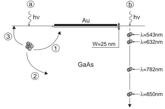
**Fig. 4.** (a) Recombination mechanisms of the charge carriers. 1: photocurrent contribution, 2: recombination in the volume, 3: recombination at the surface. (b) comparison between  $W$  and  $1/\alpha$  for different wavelengths.
