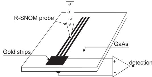
**Fig. 1.** Sample structure and principle of the experiment.
