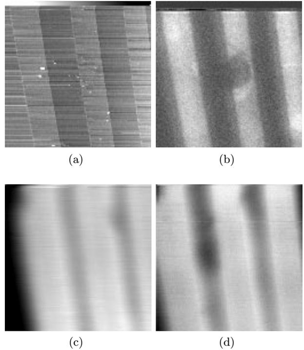
**Fig. 6.** Images with a dielectric tip and different wavelengths on the same area. The photocurrent image (b) is not “polluted” by photoconduction. (a) Topography  $30 \times 30$   $\mu\text{m}$ , (b)  $\lambda = 1.33$   $\mu\text{m}$ , (c)  $\lambda = 782$  nm, (d)  $\lambda = 632$  nm.
