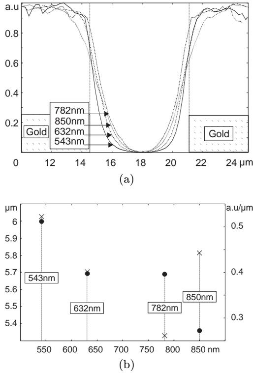
**Fig. 3.** Resolution of the photocurrent with respect to the wavelength. (a) Cross-section of the photocurrent over the gold strips, (b) slope ( $\bullet$ , right scale) and FWHM ( $\times$ , left scale) of the photocurrent over the non-metallized area *vs.* wavelength.
