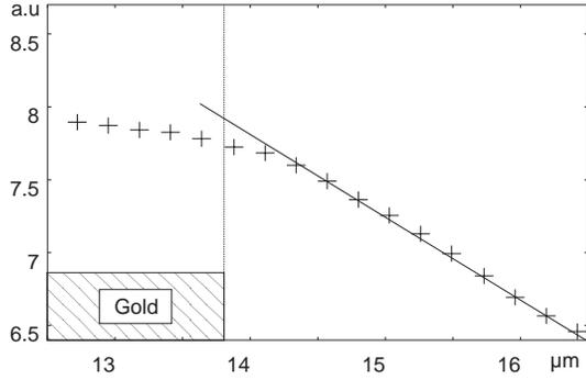
**Fig. 5.** Logarithm of the photocurrent with respect to the lateral distance for  $\lambda = 850$  nm. The slope gives  $L = 1.76$   $\mu\text{m}$  for the diffusion length.
