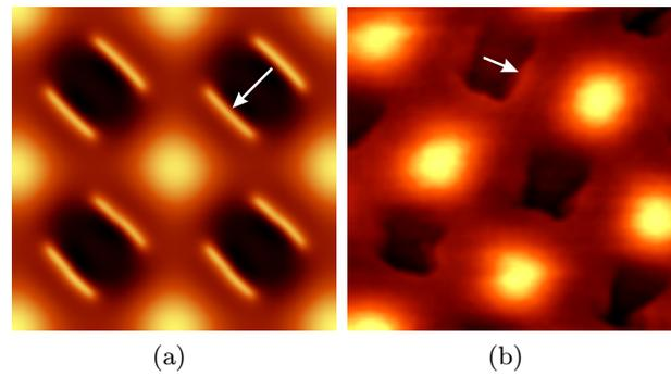
**Fig. 4.** Edge enhancement (white arrows) in both theoretical and experimental images,  $\lambda = 850 \text{ nm}$ , in both image the period of the holes is  $600 \text{ nm}$ . (a) Theoretical ( $1.2 \times 1.2 \mu\text{m}$ ), (b) experimental ( $1.5 \times 1.5 \mu\text{m}$ ).
