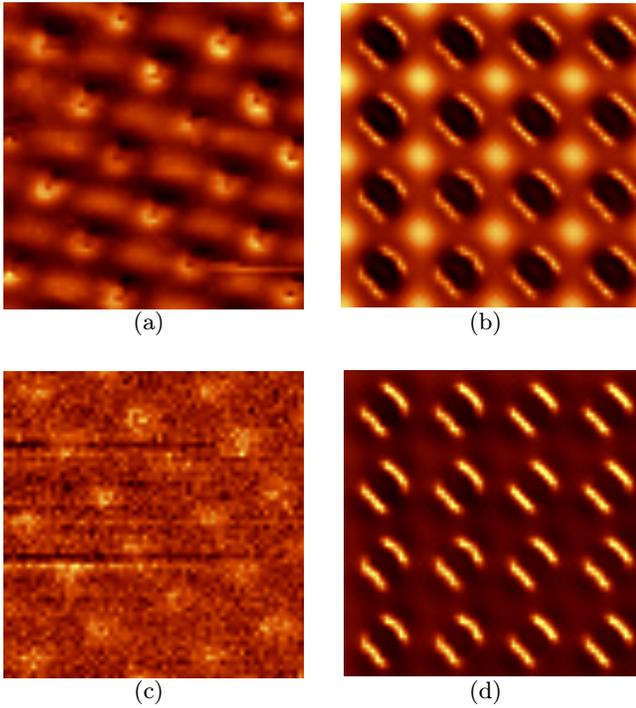
**Fig. 6.** Experimental and theoretical images on the left and on the right of the limit  $na$ . (a)  $\lambda = 850$  nm,  $3 \times 3 \mu\text{m}$ , (b)  $\lambda = 850$  nm, computed image, (c)  $\lambda = 925$  nm, (d)  $\lambda = 925$  nm, computed image.
