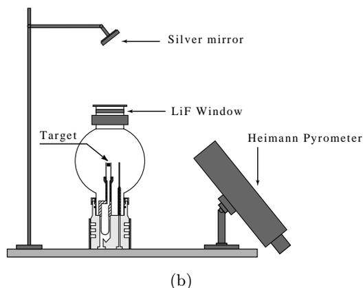
**Fig. 1.** Schematic diagram of the reactor. For carbon nanotube production the mixture of powdered graphite and catalysts is put in a graphite crucible surrounded by the graphite pipe. The inset shows the arrangement for the measurement of the target temperature.
