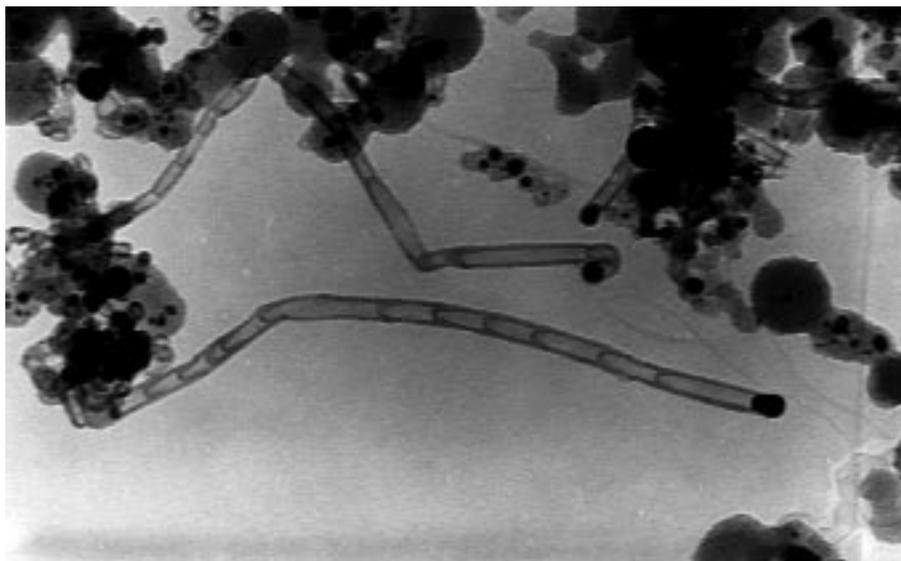
**Fig. 3.** At medium pressure (250 mbar) and for the same mixture composition as in Figure 2, we observe large amount of multi-walled nanotubes. Many of them show the presence of a catalyst nanoparticles at the end of the tube.
