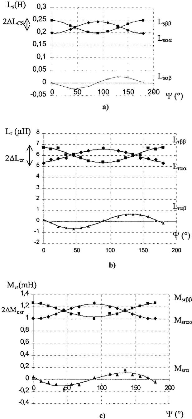
**Fig. 4.** Evolution of inductance matrix coefficients in a fixed reference frame as a function of magnetic field position ( $i_\mu = 5.55$  A): (a) stator inductances, (b) rotor inductances, (c) stator/rotor mutual inductances.
