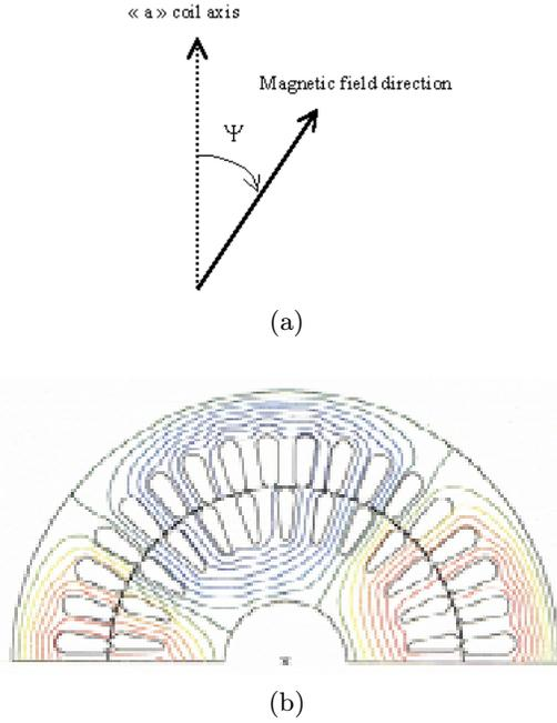
Fig. 3. (a) Field angle definition, (b) no load field distribution of the studied machine.
