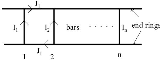
Fig. 2. Squirrel cage rotor phases representation.
