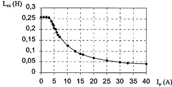
**Fig. 7.** Stator cyclic inductance evolution besides magnetising current value.
