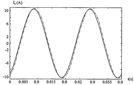
**Fig. 9.** Stator currents at nominal speed for nominal voltage supply: comparison between FEM computation (· · · · ·) and analytical results (—).
