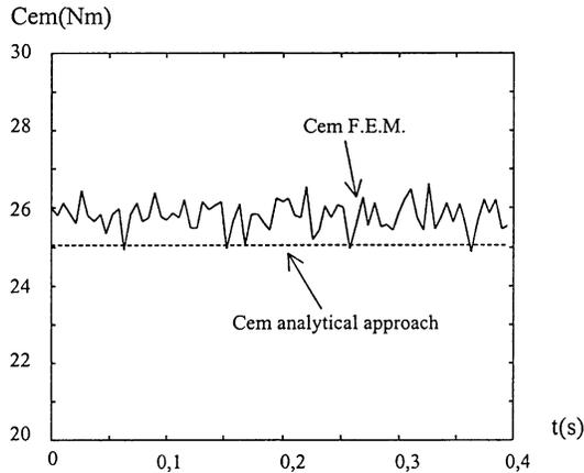
**Fig. 10.** Electromagnetic torque at nominal speed for nominal voltage supply: comparison between FEM computation (mean value = 25.8 Nm) and analytical results (25 Nm).
