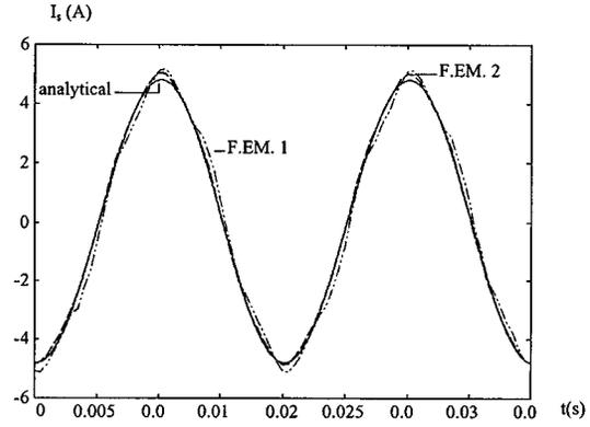
**Fig. 8.** Stator currents at no load for nominal voltage supply: comparison between analytical approach (—) and FEM computations, with (· · · · 1) and without (--- 2) rotor bar conductivity.
