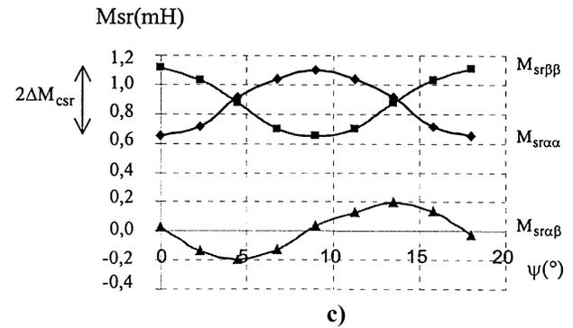
**Fig. 5.** Evolution of inductance matrix coefficients in a fixed reference frame as a function of magnetic field position, ( $i_\mu = 10$  A): (a) stator inductances, (b) rotor inductances, (c) stator/rotor mutual inductances.
