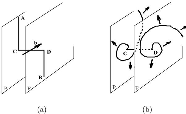
**Fig. 8.** Multiple spiral Frank-Read source. (a) Dislocations  $AC$  and  $BD$  are glissile, whereas  $CD$  is a sessile dislocation segment acting as anchorage for the potential source. (b) Glissile segments expand under stress in a spiral-shape in their own crystallographic slip planes. Each sessile jog along the dislocation line is hence a potential dislocation source, so-called Multiple spiral Frank-Read source.
