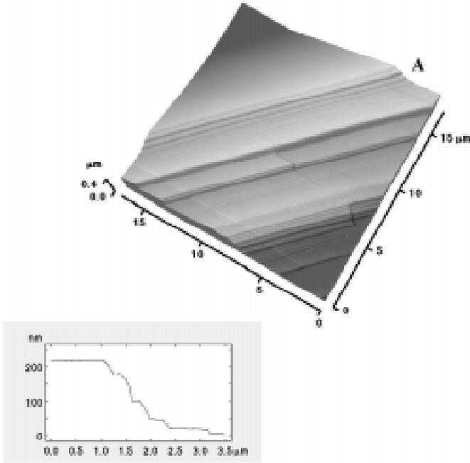
**Fig. 1.** Topographical AFM image of the fine slip line structure of a Ni based superalloy phase  $\gamma$  single crystal. The sample has been deformed up to 1.03%. A profile plot of the step structure labeled A, obtained by averaging few consecutive sections perpendicularly to the slip lines, is presented.
