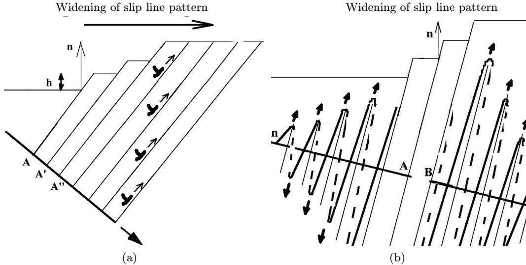
**Fig. 7.** Step structure generated at the surface resulting from the activation of various dislocation sources for (a) a movable Frank-Read source (b) a helical Frank-Read source.
