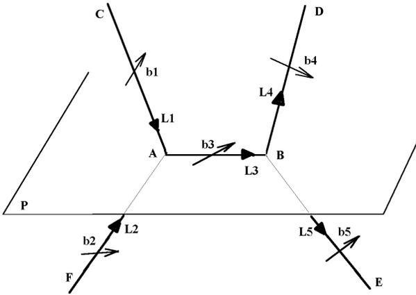
**Fig. 2.** Schematic diagram of external dislocation network around a potential dislocation source  $A-B$ . The associated slip plane is labeled  $P$ . Each dislocation ( $i$ ) is symbolized by its line direction  $L_i$  and Burgers vector  $b_i$ .
