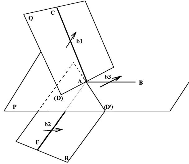
**Fig. 3.** Dislocations  $CA$  and  $FA$  are restricted to move in planes  $Q$  and  $R$  respectively. Point  $A$  is the intersection of lines  $D$  and  $D'$  and acts therefore as pinning point for the dislocation source. A similar behaviour occurs at point  $B$ .
