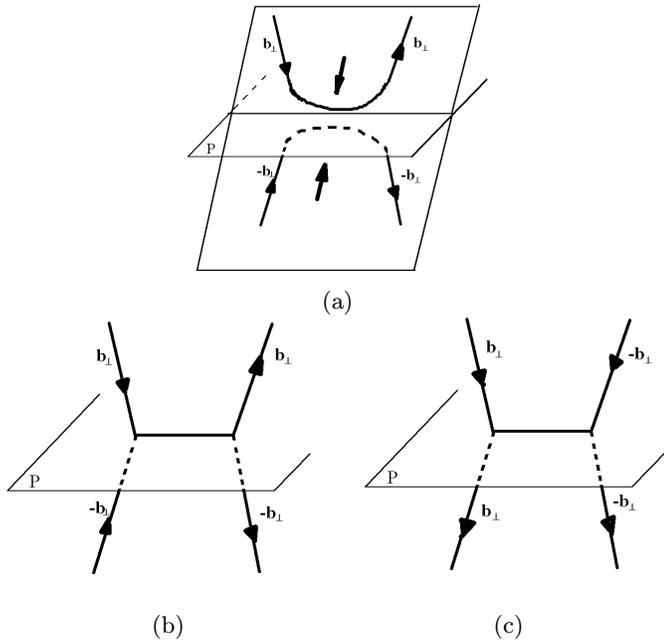
**Fig. 4.** Configuration  $\mathbf{b}_1 = \mathbf{b}_4$  and  $\mathbf{b}_2 = \mathbf{b}_5$ , resulting from the recombination of dislocations at the intersection of their slip planes. Each dislocation is here represented by its Burgers vector component perpendicular to plane  $P$  and an arrow indicates the direction of the slip line: (a) origin of studied dislocation network; (b) schematic configuration; (c) equivalent configuration by FSRH consideration.
