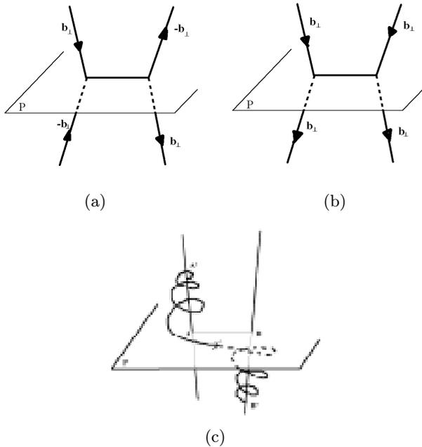
**Fig. 6.** Activation of *helical Frank-Read source*. (a) Configuration of external dislocation network issued from dislocation interaction with the further creation of junction in-between. (b) Equivalent configuration by FRSH convention. (c) Behaviour of the initial dislocation segment  $A-B$  under stress. As *movable Frank-Read source*, the dislocation expands and wraps up around  $A$  and  $B$  points, but on both sides of slip plane  $P$ , which prevents subsequent recombination.
