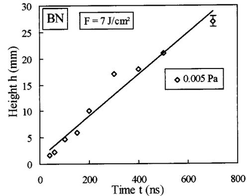
**Fig. 7.** Evolution of height  $h$  (mm) reached by the front (BN target) with delay time  $t$  (ns) at  $7 \text{ J/cm}^2$  under vacuum: free motion.
