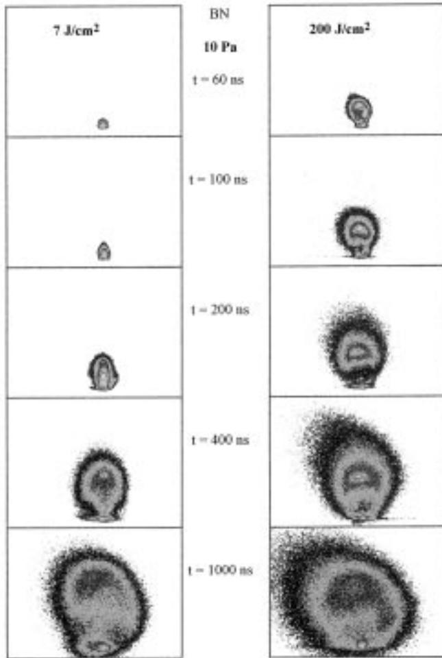
**Fig. 4.** Evolution of the plume created above a BN target, performed at 10 Pa ( $N_2$ ) as a function of the laser fluence: 7 and  $200 \text{ J/cm}^2$  (delays  $t$  from 60 to 1000 ns).
