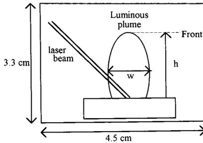
Fig. 2. Schematic representation of the region observed by the ICCD camera;  $h$  and  $w$  are respectively the height of the luminous front and the width of the plume. The laser beam comes from the left with an incidence of  $45^\circ$ .
