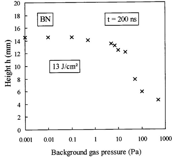
**Fig. 9.** Height  $h$  reached by the luminous front at  $t = 200 \text{ ns}$  above a BN target ( $13 \text{ J/cm}^2$ ) as a function of pressure in the cell: from residual background pressure up to  $500 \text{ Pa}$  ( $\text{N}_2$ ).
