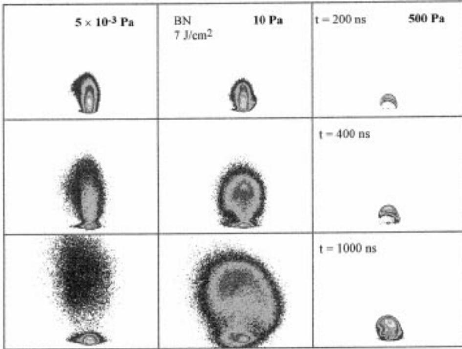
**Fig. 6.** Evolution of the plume created above a BN target, performed at  $7 \text{ J/cm}^2$  as a function of pressure in the cell: under vacuum ( $5 \times 10^{-3} \text{ Pa}$ ), at 10 and 500 Pa ( $\text{N}_2$ ) (delays  $t$ : 200, 400, 1000 ns).
