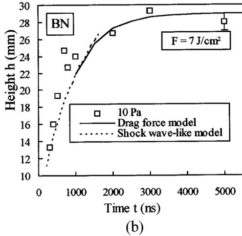
**Fig. 8.** Evolution of height  $h$  (mm) reached by the front (BN target) with delay time  $t$  (ns) at  $7 \text{ J/cm}^2$  at  $10 \text{ Pa}$  ( $\text{N}_2$ ): (a)  $h$  up to  $1 \text{ cm}$ : free motion; (b)  $h > 1 \text{ cm}$ : dotted curve = the shock wave model fit; full curve = the drag force model fit.
