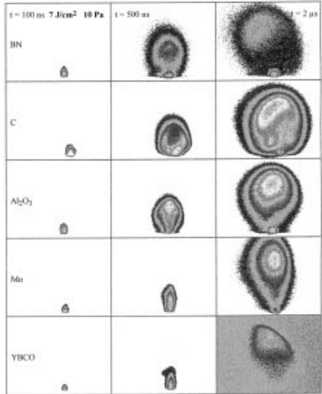
Fig. 3. Images of the plumes created above the five targets, performed at  $7 \text{ J/cm}^2$ , 10 Pa ( $\text{N}_2$ ) (size:  $3.3 \times 4.5 \text{ cm}^2$  (height  $\times$  width)) for three delays  $t$  after the beginning of the laser pulse (duration 20 ns). The target is at the bottom of each image.
