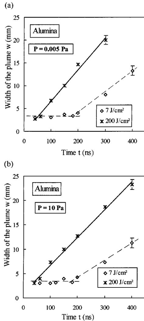
**Fig. 5.** Evolution of width  $w$  (mm) of the plume (alumina target) with delay time  $t$  (ns) and with laser fluence (7 and  $200 \text{ J/cm}^2$ ): (a) at  $5 \times 10^{-3}$  Pa (vacuum); (b) at 10 Pa ( $N_2$  gas).
