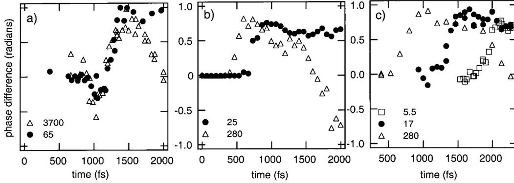
**Fig. 1.** Time-resolved phase measurements for three pulse durations and various laser irradiances in TW/cm<sup>2</sup>. (a) Pump pulse duration of 0.16 ps; (b) 0.76 ps; (c) 2.2 ps.
