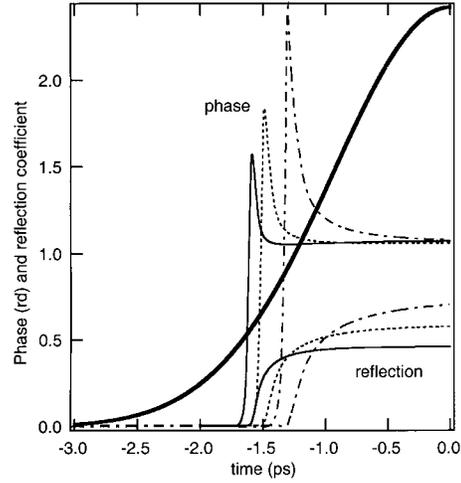
**Fig. 2.** Time evolution of the phase and the amplitude of the reflected probe pulse for 2.2 ps duration laser pulse as a function of the electron-phonon momentum transfer collision rate. Dashed-dotted line:  $\nu = 10^{15} \text{ s}^{-1}$ , dotted line:  $\nu = 2 \times 10^{15} \text{ s}^{-1}$ , solid line:  $\nu = 3 \times 10^{15} \text{ s}^{-1}$ . The laser irradiances is  $20 \text{ TW}/\text{cm}^2$ . *p*-polarised probe light at 400 nm.
