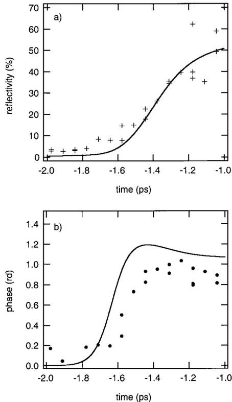
**Fig. 5.** Time-resolved reflectivity (a) and phase (b) measurements for 2.2 ps pump pulse duration and  $1.7 \times 10^{13} \text{ W/cm}^2$  irradiance for *p*-polarised light. The solid line is the result of the model described in the text.
