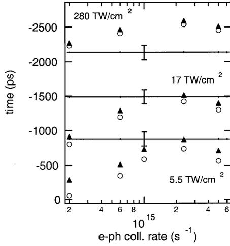
**Fig. 3.** Calculated breakdown times (with respect to the peak of the 2.2 ps duration laser pulse) as a function of the electron-phonon momentum transfer collision rate. Filled symbols: 3 eV; Open symbols: 1 eV electron temperature. From top to bottom, the laser irradiances are 280, 17, and 5.5 TW/cm<sup>2</sup>. Horizontal lines are the experimental results with error bars.
