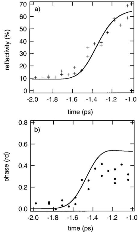
**Fig. 4.** Time-resolved reflectivity (a) and phase (b) measurements for 2.2 ps pump pulse duration and  $1.7 \times 10^{13} \text{ W/cm}^2$  irradiance for *s*-polarised light. The solid line is the result of the model described in the text.
