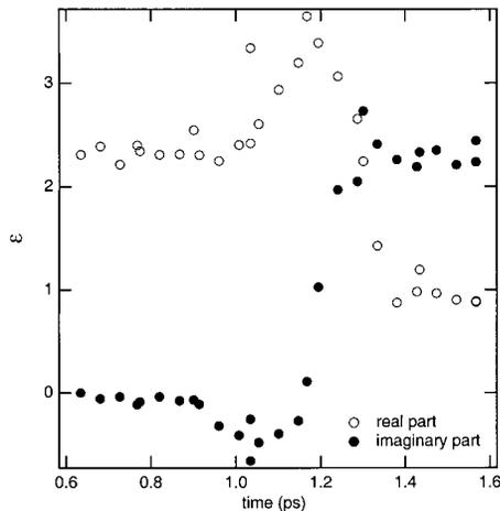
**Fig. 6.** Time-resolved real and imaginary part of the dielectric constant of silica during breakdown for 0.16 ps pump pulse duration and  $6.5 \times 10^{13} \text{ W/cm}^2$  irradiance.
