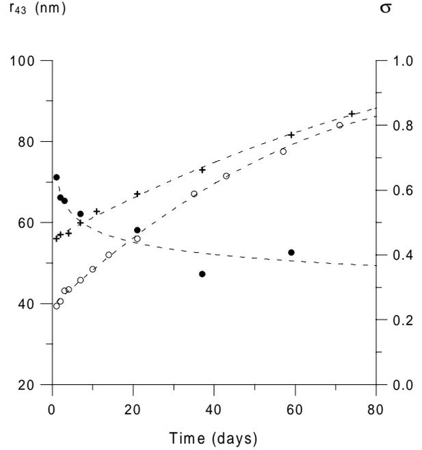
**Fig. 6.** Variation of the mean radius  $r_{43}$  ( $\circ$ ) and the polydispersity  $\sigma$  ( $\bullet$ ) with time during the ageing of the hexadecane in water emulsion. Also plotted is the apparent hydrodynamic radius ( $+$ ) determined at  $90^\circ$  by dynamic light scattering: the estimations are heavily overestimated for the smallest and most polydisperse emulsions.
