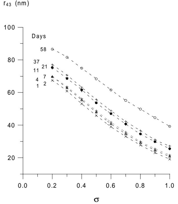
**Fig. 4.** Combinations of the values of radius and polydispersity ( $r_{43}, \sigma$ ) which lead to the best fit for each static light scattering experiment (the dashed lines are guides for the eye). It is virtually impossible here, to ascertain the values of both  $r_{43}$  and  $\sigma$ .
