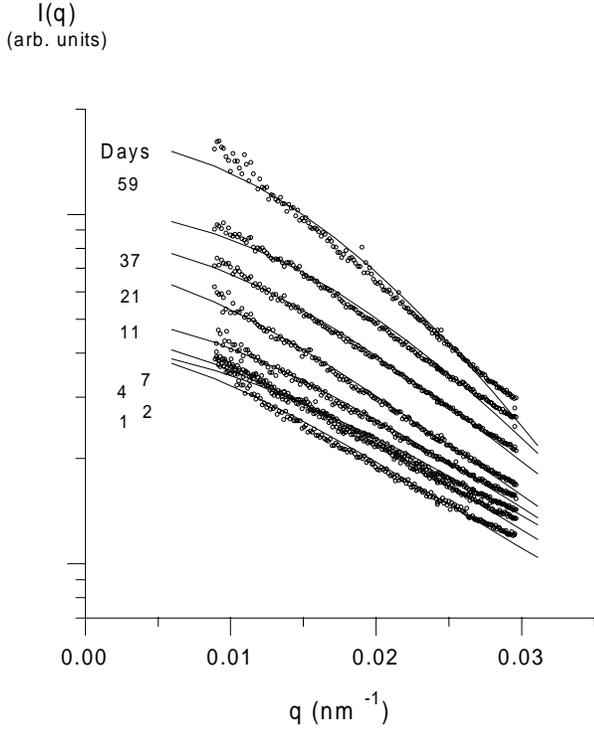
**Fig. 3.** Evolution of the form factor (light intensity *versus* scattering wave vector) during the ageing of a 10% vol/vol *n*-hexadecane/water emulsion. Curves are best fit to theoretical values. The large increase of the scattered intensity expresses the growth of the droplets.
