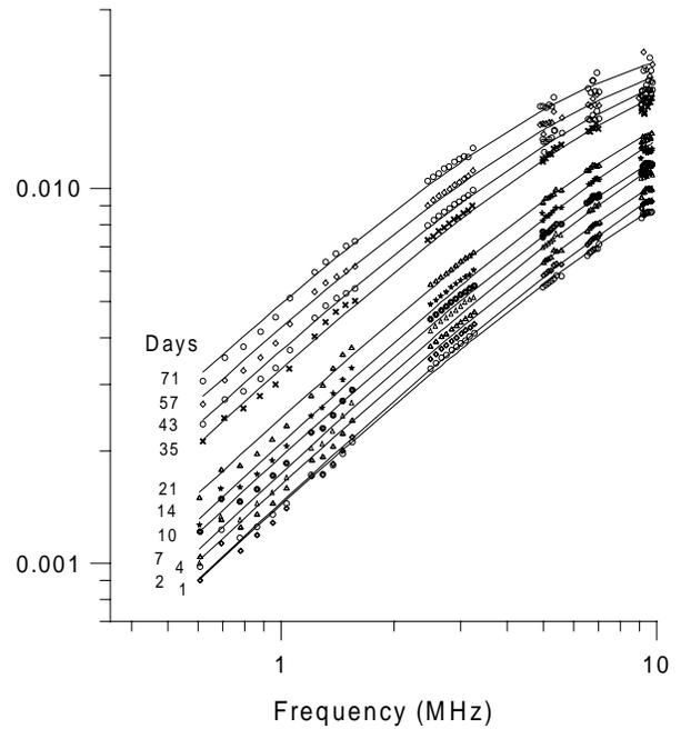
**Fig. 1.** Evolution of the ultrasonic attenuation spectra during the ageing of a 10% vol/vol *n*-hexadecane/water emulsion. Curves are best fit to theoretical values. A variation of 1 nm of the apparent radius can easily be distinguished.
