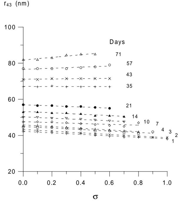
**Fig. 2.** Combinations of the values of radius and polydispersity  $(r_{43}, \sigma)$  which lead to the best fit for each ultrasonic attenuation spectrum (the dashed lines are guides for the eye). The estimation of the volume average radius  $r_{43}$  is fairly insensitive to the polydispersity, which makes it a good parameter for characterizing emulsions.
