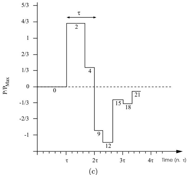
**Fig. 1.** Space-time diagram of a square pulse propagating in a substrate A with a coating B whose shock impedance is higher than the substrate's one (a), corresponding states on the (pressure-particle velocity) plane (b) and sketch of the stress history generated at the interface (c).
