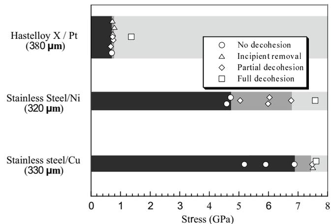
**Fig. 6.** Peak values of traction generated at the interface of systems determined by numerical simulation and corresponding damage observed experimentally on the coating allowing to read the debonding threshold of each system.
