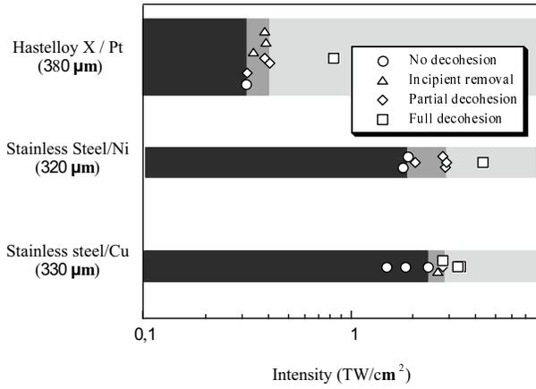
**Fig. 4.** Experimental observation of the damage produced on the tested systems *versus* the incident laser intensity.
