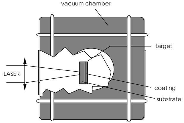
**Fig. 2.** Experimental set-up used to determine the debonding threshold for various systems.
