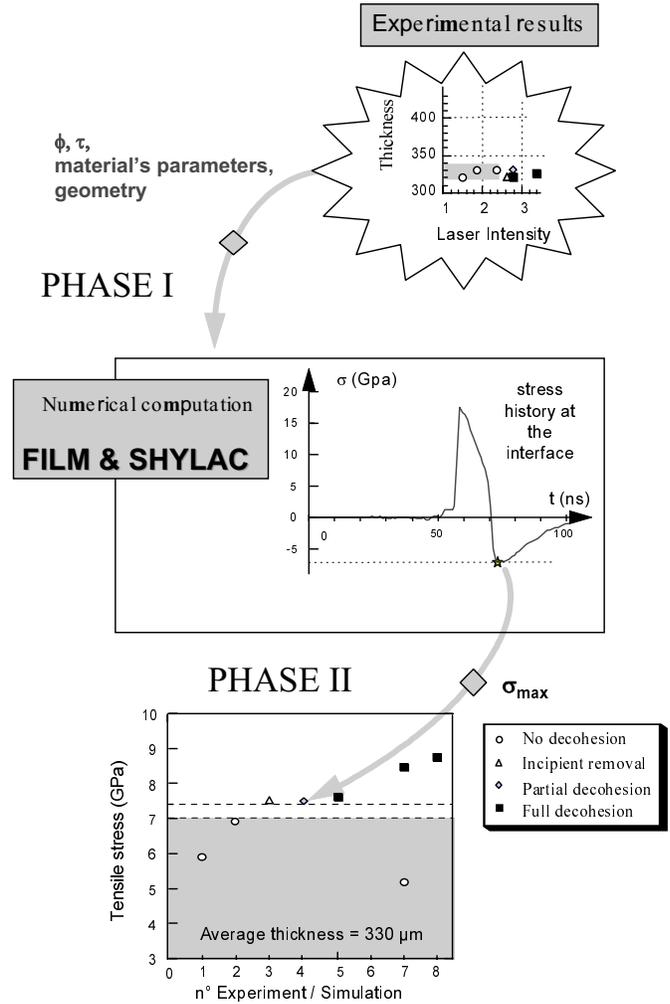
**Fig. 5.** Sketch of the principle of determination of the traction peak values at the interface by numerical simulation of the experiments using FILM and SHYLAC codes.
