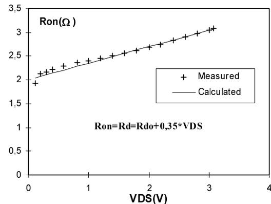
**Fig. 3.** Typical variations of the on-state resistance with respect to the drain bias, at  $V_{GS} = 10$  V.
