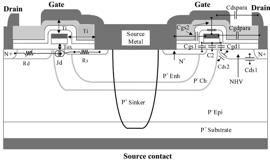
**Fig. 1.** Schematic cross-section (AA') of two elementary fingers of the SHF radio frequency LDMOS transistor.
