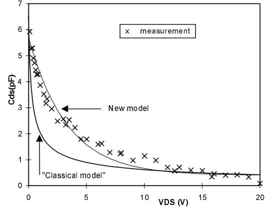
**Fig. 11.** Variations of the drain-source capacitance with respect to the drain-source voltage.
