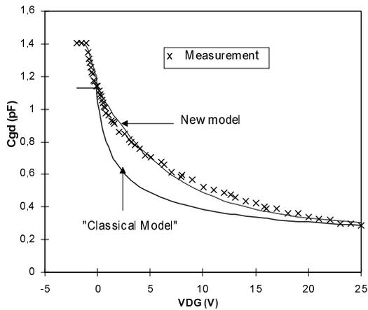
**Fig. 10.** Variations of the gate-drain capacitance with respect to the drain-gate voltage at  $V_{GS} = 0$  V.
