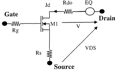
**Fig. 4.** Equivalent circuit in the static mode of the SHF LDMOS.
