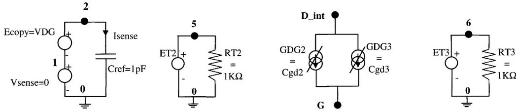
**Fig. 7.** Modelling of the capacitances  $C_{gd2}$  and  $C_{gd3}$  in PSPICE.
