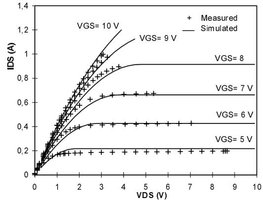
**Fig. 12.** Static output characteristics of the SHF LDMOS transistor.
