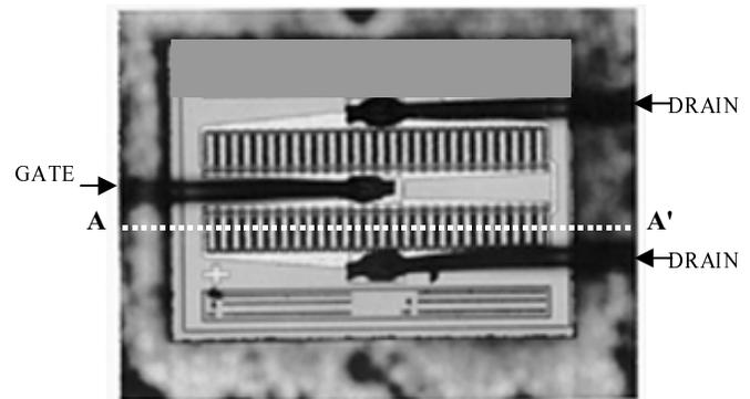
**Fig. 2.** Microphotography of the SHF LDMOS transistor (two cells, 3 W at 2 GHz).
