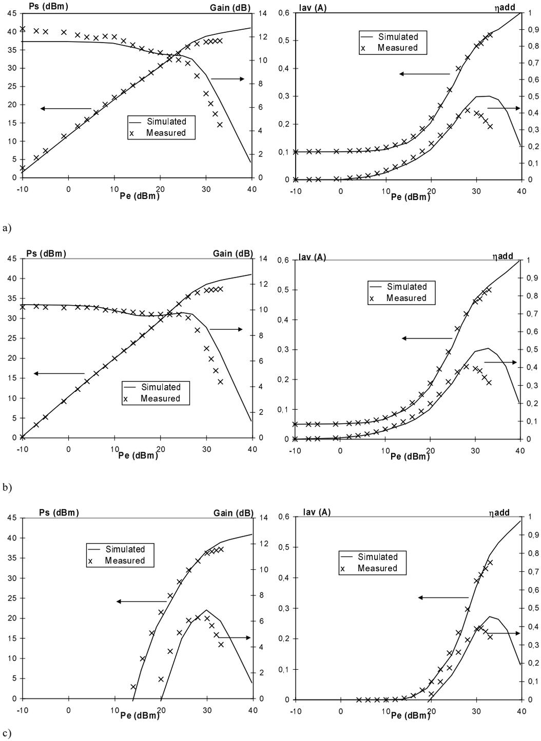
**Fig. 14.** Transfer characteristic  $P_s(P_e)$ , power gain  $G(P_e)$ , mean current  $I_{av}(P_e)$  and power added efficiency  $\eta_{add}(P_e)$ : (a)  $I_{DS0} = 100$  mA, (b)  $I_{DS0} = 50$  mA, (c)  $I_{DS0} = 0$  mA.  $E_d = 26$  V, the working frequency is 2 GHz.
