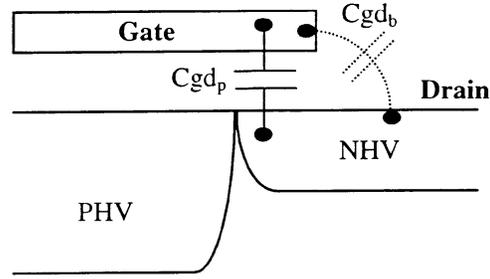
**Fig. 6.** Components of the capacitance  $C_{gd1}$ .
