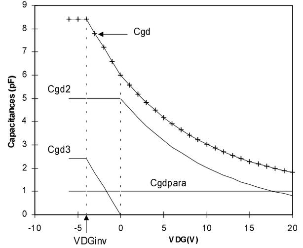
**Fig. 5.** Typical variation of the “reverse” capacitance  $C_{gd}$ .
