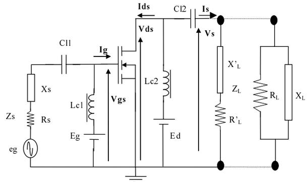
**Fig. 13.** Radio Frequency amplifier circuit as it is implemented in PSPICE.
