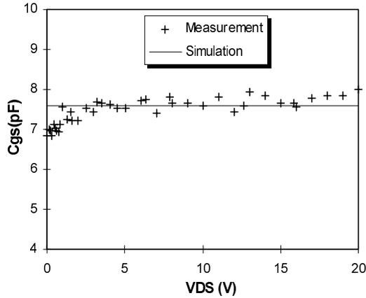
**Fig. 9.** Variations of the gate-source capacitance with respect to the drain-source voltage.
